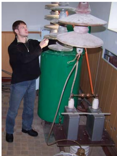
Fig. 1. Insulator testing unit
