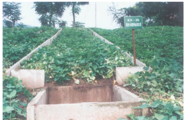
Runoff plot in Kaixian of Chongqing (purple soil, rape- Ipomoea batatas intercropping and 25° in gradient)
