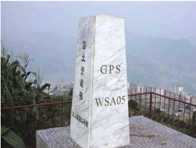
Observation pier of A-level GPS control network
