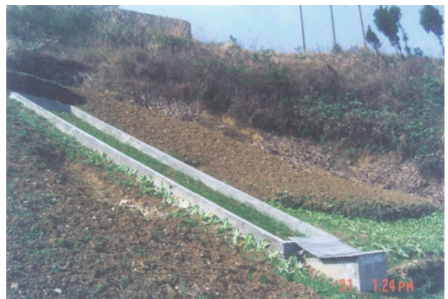
Runoff plot of Wanzhou, Chongqing (lime soil, corn- Ipomoea batatas intercropping, 25° in gradient). Photo by Huang Zhenli
