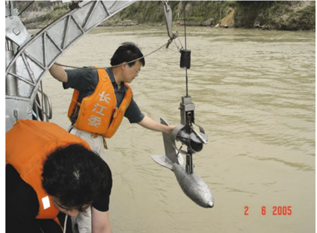
Collecting water samples from the mainstream of the Yangtze at the construction site
