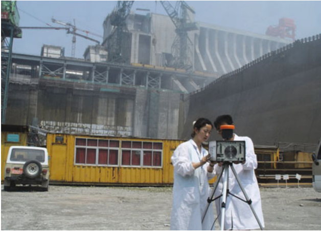
Monitoring flying dust in the construction pit of the third phase coffer dam (photo by Huang Zhenli)
