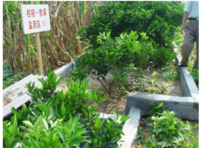
There are 48 additional runoff areas, with different soil types, planting modes and gradients to monitor the non-point pollution load of slope land. The picture shows the runoff plot (yellow soil, orange-grazing grass intercropping and 5° of gradient) at Longtanping village, Taipingxi Town, Yiling District of Yichang City. Photo by Huang Zhenli
