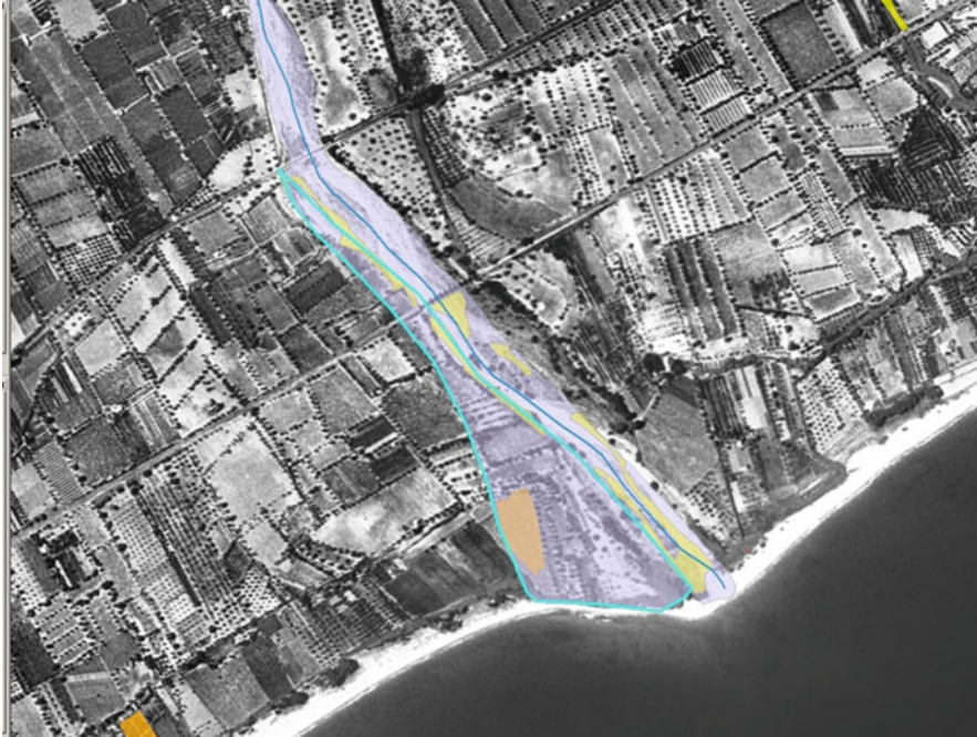
Fig. 3 An example of photo-image obtained from 1956 with present riparian land uses shown above as coloured polygons used to assess the land use on river banks and floodplain areas in Catalan rivers
