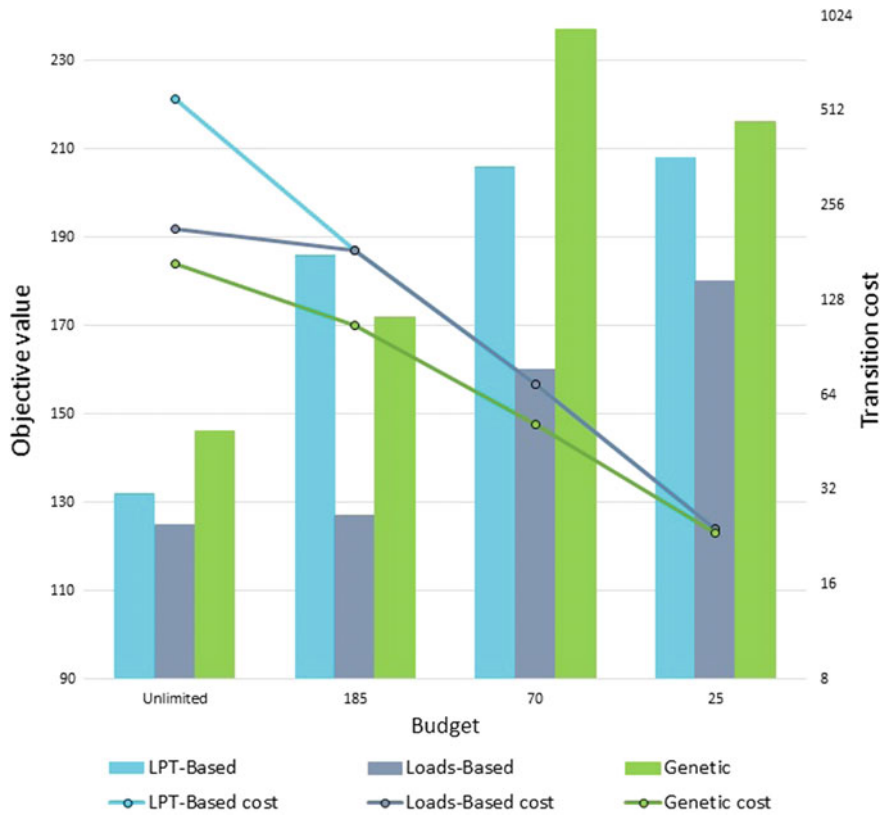
Fig. 6 Results for \min C_{max} with m/2 added machines and variable budget
