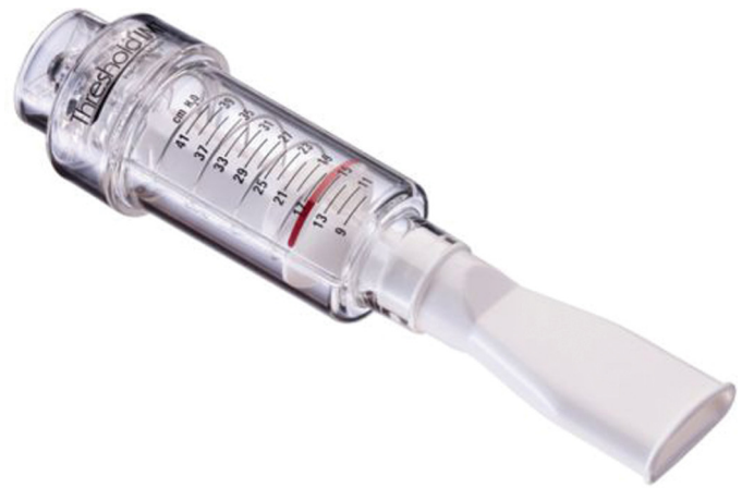
Fig. 12.12 The Threshold inspiratory muscle trainer (IMT) incorporates a flow-independent one-way valve to ensure consistent resistance and features an adjustable pressure threshold setting in cmH_2O . When the patient breathes through the Threshold IMT, a spring-loaded valve provides a resistance that exercises respiratory muscles through conditioning.
