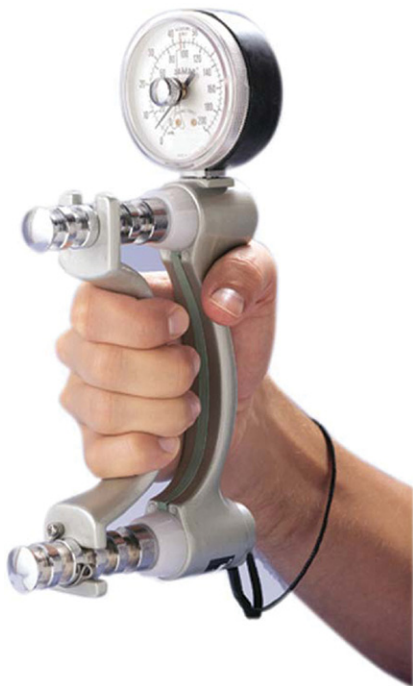
Fig. 12.11 The Jamar dynamometer is the classical tool for measuring handgrip force. This dynamometer has an adjustable top-workbench to fit different hand sizes and is a hydraulic isometric hand dynamometer with readings in kilograms (kg) with 2 kg gradation.
