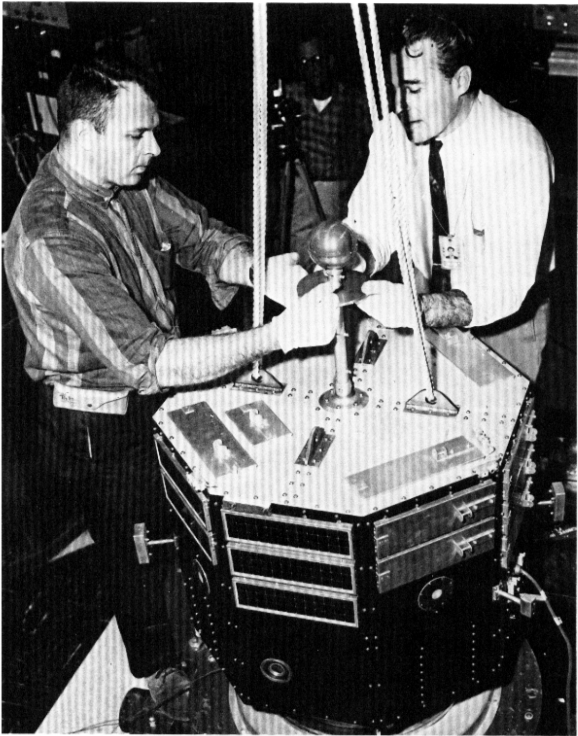
Silicon solar cells were a durable, compact, lightweight source of electric power for this Explorer space satellite.
