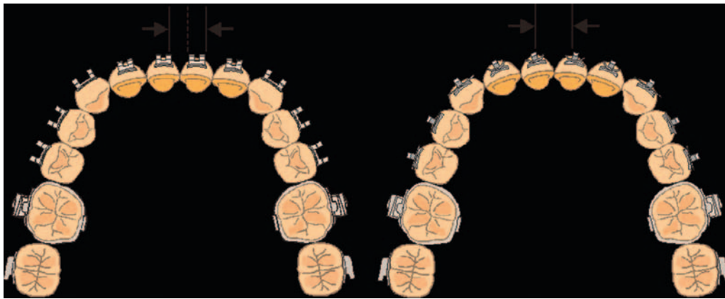
Fig. 11.2 Forty-eight percent increased interbracket space compared to twin brackets. Left: Twin brackets Right: Alexander bracket with wings
