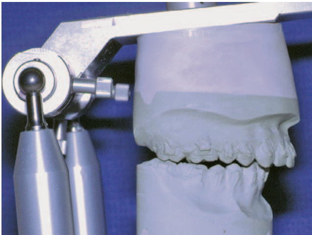
Fig. 16.1.23 The SAM Mandibular Position Variator is designed for repositioning the condylar elements during splint fabrication. Each condylar element has two gears (one each in the X and Y planes), which are calibrated in millimeters such that when activated in either the X or Y plane, the maxillary model moves either posterior or superior, respectively. This gives a corresponding representation of anterior or inferior mandibular movement. For distraction, one set of mounted presurgical models was transferred from a SAM 3 articulator to the variator.
