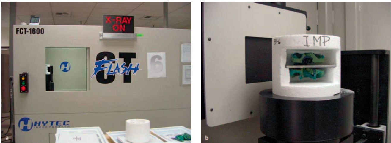
Fig. 13.2 The impressions are scanned by a CT-scanner (a) as they rotate in a styrofoam holder in front of an amorphous silicon x-ray sensor (b).
