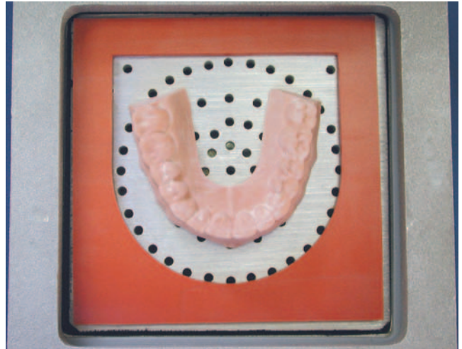
Fig. 15.17 A larger vacuum condensing gasket necessary to accommodate the increased dimensions of a full-arch cast.
