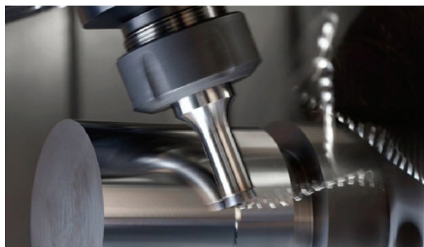
Figure 1.23 Spinning tool jointly developed by Mori Seiki and Kennametal
