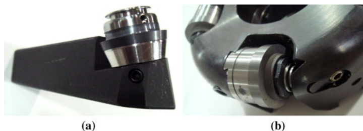
Figure 1.22 (a) Self-propelled single-point tool, and (b) milling tool
