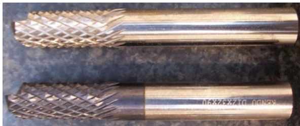
Figure 2.1 Milling tool for routing carbon-fibre-reinforced plastics, by Kendu ® , made of sub-micrograin tungsten carbide ( top ), and with TiAlN coating applied by Metal Estalki ® ( bottom )
