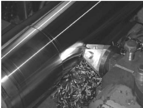
Figure 1.12 Hard “skiving” turning
