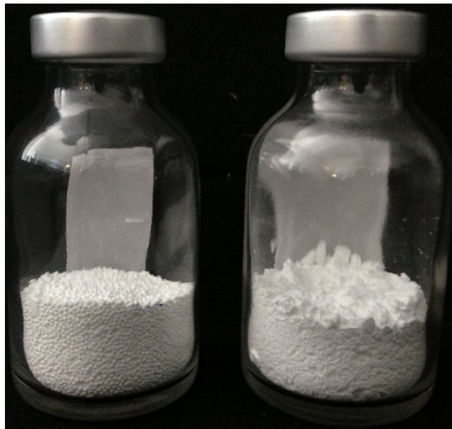
Figure 10.5 Soft agglomerates of amikacin. Right: original spray dried powder; left: the same powder after agglomeration
