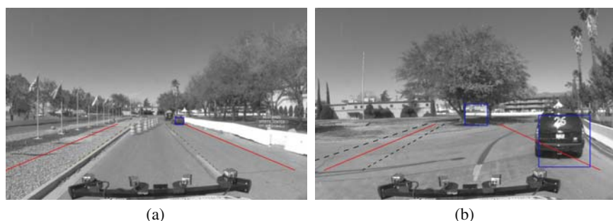
Fig. 28. Results of explicit vehicle detection in the collision. (a) DARPA chase vehicle detected. (b) Last frame: Skynet is detected. Trees and clutter in the background also generate false positives during the sequence. In the intersection there are no lane markings so lane estimate confidence cannot be used to exclude the false detections.
