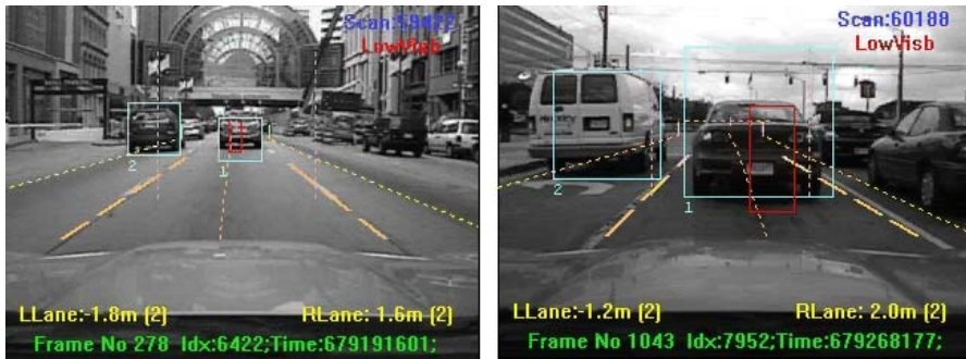
Fig. 12. Delphi/Mobileye radar/vision fusion with lane detection and in-path targets.
