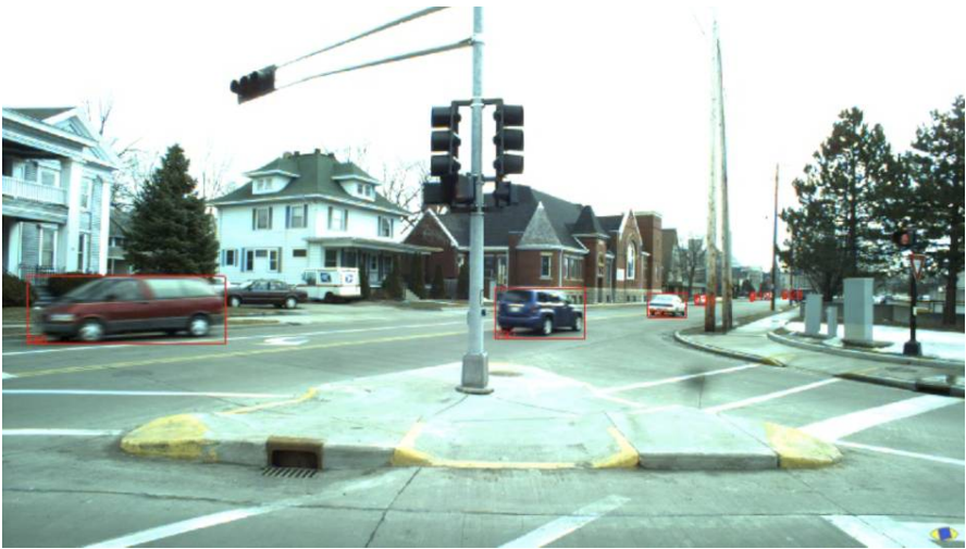
Fig. 8. Lateral system algorithm results (detected vehicles are marked red).
