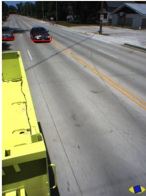
Fig. 9. Rear view system algorithm results (detected vehicles are marked in red).
