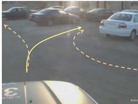
Fig. 16. During NQE B, Odin did not pull into the parking spot by the direct path (solid line). Instead, Odin pulled to the left (dashed line), circling the parked cars and eventually entered the space.
