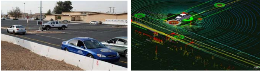
Fig. 23. Area A “circles of death.” XAV-250 waits to merge into traffic (left). MIT viewer showing the RNDF course with obstacles derived from the radars and Velodyne point cloud (right).
