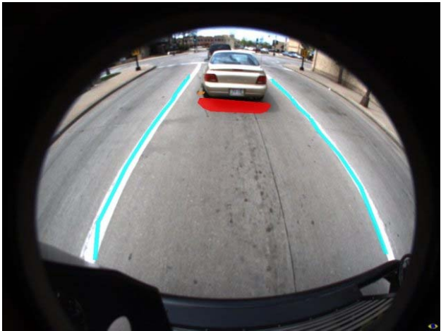
Fig. 7. A sample frame showing typical obstacle and lane detection.
