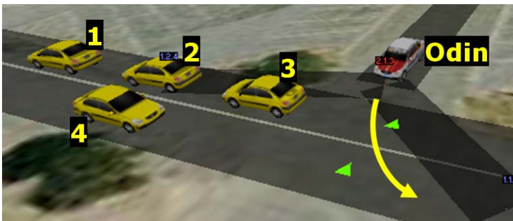
Fig. 15. A merge in NQE course A with an occluded vehicle (vehicle 4)
