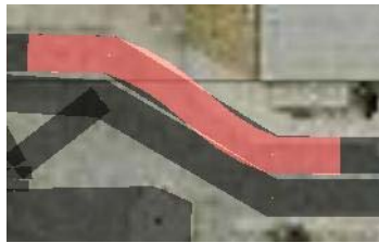
Fig. 19. Report Lane Position overlay for lane 8.1 of the UCE RNDF where Odin clipped a curb
