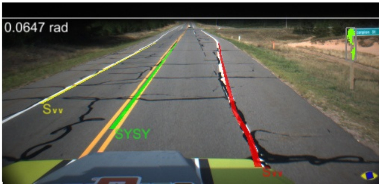
Fig. 6. Results of lane detection algorithm projected on the original image. From right to left, the red line represents a right boundary, green a left boundary, and yellow a far left boundary. In this image, the right line is detected although it is not a complete line.
