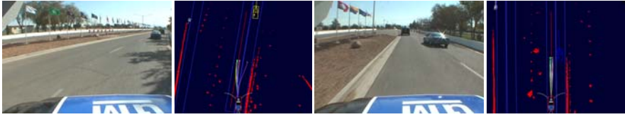
Fig. 8. Performing a lane change reliably and safely. Here, Boss changed lanes because another robot’s chase vehicle was traveling too slowly in its original lane.
