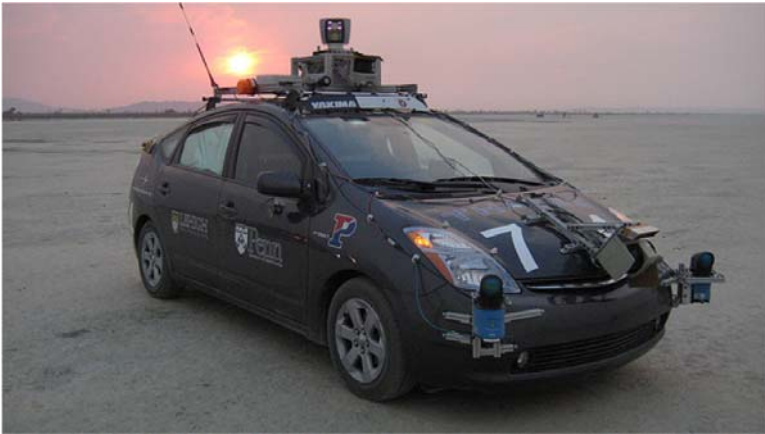
Fig. 1. Little Ben is a Toyota Prius hybrid vehicle modified for drive-by-wire operation with an onboard array of sensors and computers.
