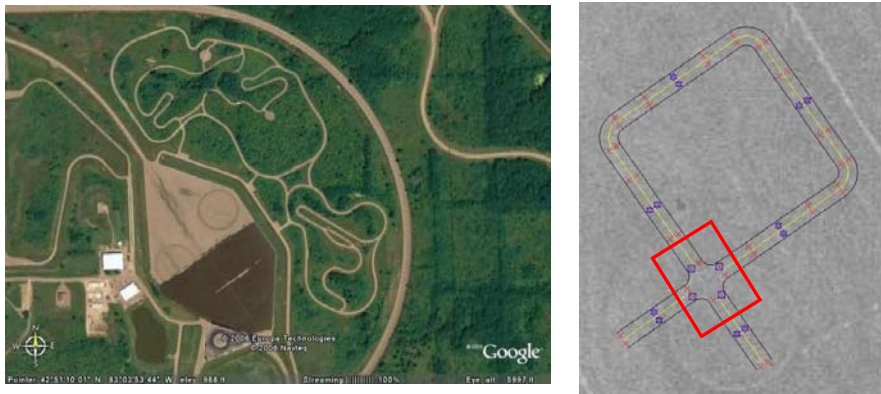
Fig. 16. Michigan Proving Grounds vehicle dynamics test Area, precision steering course, and Site Visit Course. Lane markings for the Site Visit course were laid out using reflective highway construction tape. The intersection area contained in the red rectangle is discussed in the next figure.
