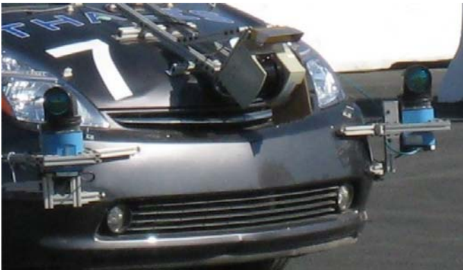
Fig. 7. Sensors mounted on the hood of Little Ben.
