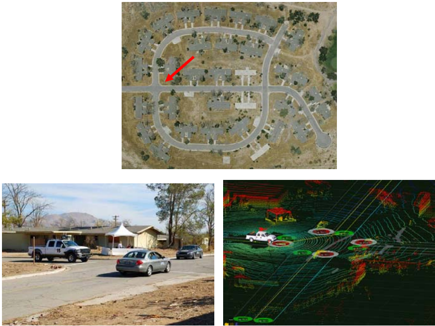
Fig. 22. Area C – intersection logic and dynamic re-planning. Aerial photo of Area C course (top); red arrow indicates the intersection depicted in figures below. XAV-250 successfully exhibits advanced traffic behavior (bottom left). MIT viewer rendering of the RNDF and tracked cars at the intersection (bottom right).
