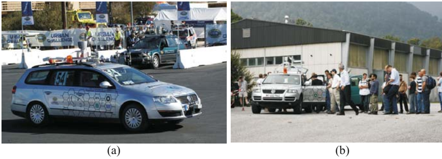
Fig. 1. The two vehicles our approach was tested with. (a) The VW-Passat of Darpa Urban Challenge finalist Team AnnieWay (b) The VW-Touareg MuCAR-3 (Munich Cognitive Autonomous Robot, 3rd generation), a C-Elrob 2007 Champion. Both vehicles are equipped with a 360 degree Velodyne-LIDAR as primary sensor scanning its environment at 10 Hz using 64 laser beams.
