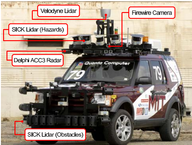
Fig. 9. MIT's 'Talos', a Land Rover LR3 featuring five Point Grey FireFly cameras, 15 Delphi ACC3 radars, 12 Sick LMS-291 lidars and a Velodyne HDL-64 lidar.
