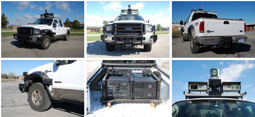
Fig. 5. Collage of XAV-250 images revealing key elements of the external hardware. Truck overview (top left); protective frontal exoskeleton with 3 embedded in-line ACC radars and single centered BUA radar underneath (top center); rear view showing GPS mast on rooftop and protected pair of ACC and BUA radars (top right); side exoskeleton with ACC and BUA radars (bottom left); climate controlled and shock isolated box containing computing cluster (bottom center); and lidar and vision systems (bottom right), with Velodyne at apex, Riegl lidars left and right, and cameras hidden within the Velodyne tower and behind the windshield glass.
