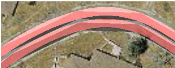
Fig. 7. Example of the splined lane positions (bright overlays) output matching the actual roads in the aerial imagery. The road displayed is segment 11 of the UCE RNDF.
