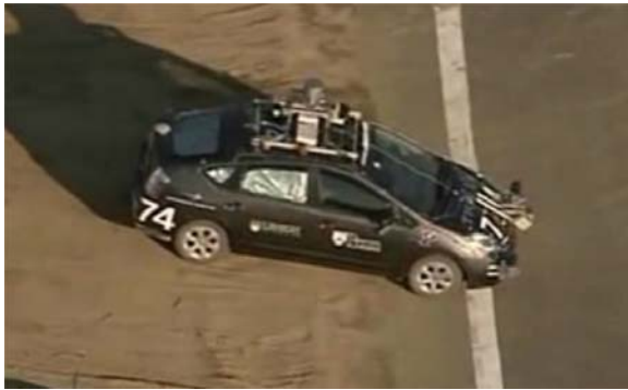
Fig. 22. Little Ben temporarily stalled on the transition from the Outback to Phantom Road East. The steep pitch of the transition resulted in the road surface being falsely classified as an obstacle.
