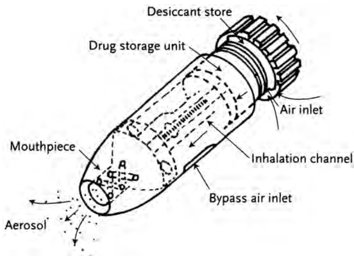
Figure 10.8 The essential components of a Turbuhaler
