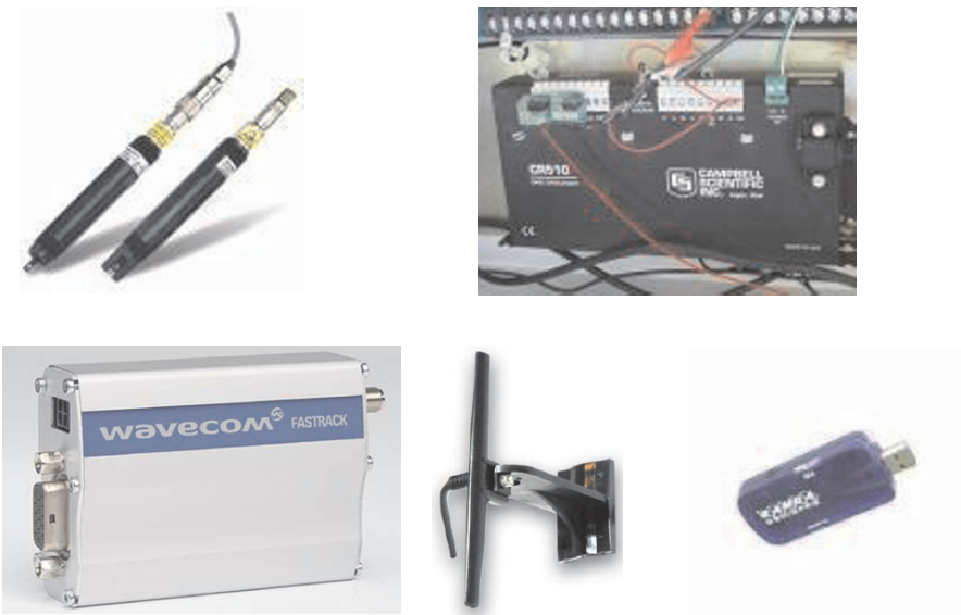
Figure 2. Components of an automatic emergency warning unit proposed to be installed at the transboundary potential emergency points in Armenia
