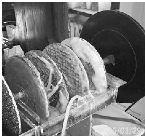
Figure 4. Photos of the biofilm in the denitrification part of the RBS reactor.
