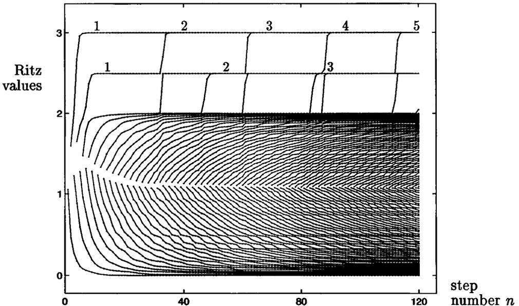
Figure 36.3. Continuation to 120 steps of the Lanczos iteration. The numbers indicate multiplicities of the Ritz values. Note the appearance of four “ghost” copies of the eigenvalue 3.0 and two “ghost” copies of the eigenvalue 2.5.
