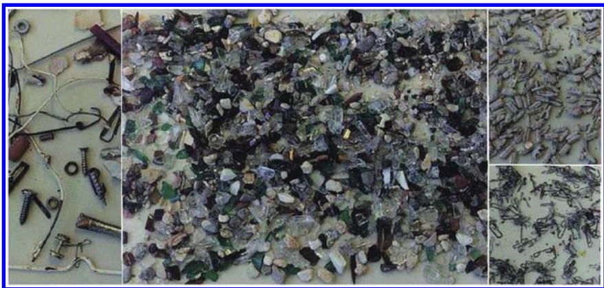
FIGURE 12.22 Particles typically separated by heavy weight coarse cleaner.
