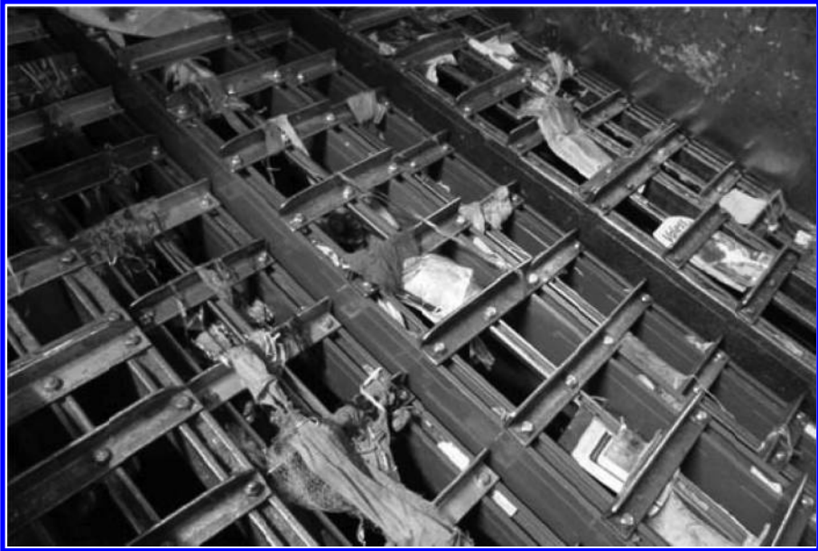
FIGURE 12.12 Photo of a ballistic separator used for separating larger board and packaging materials from graphic papers.
