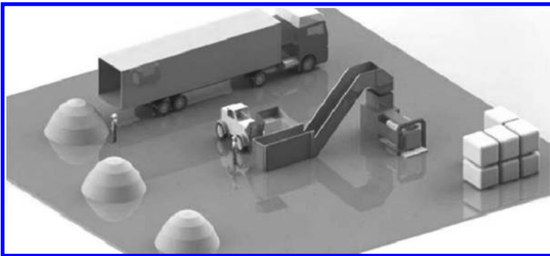
FIGURE 12.8 Dry recovered paper sorting plant: pressing station.
