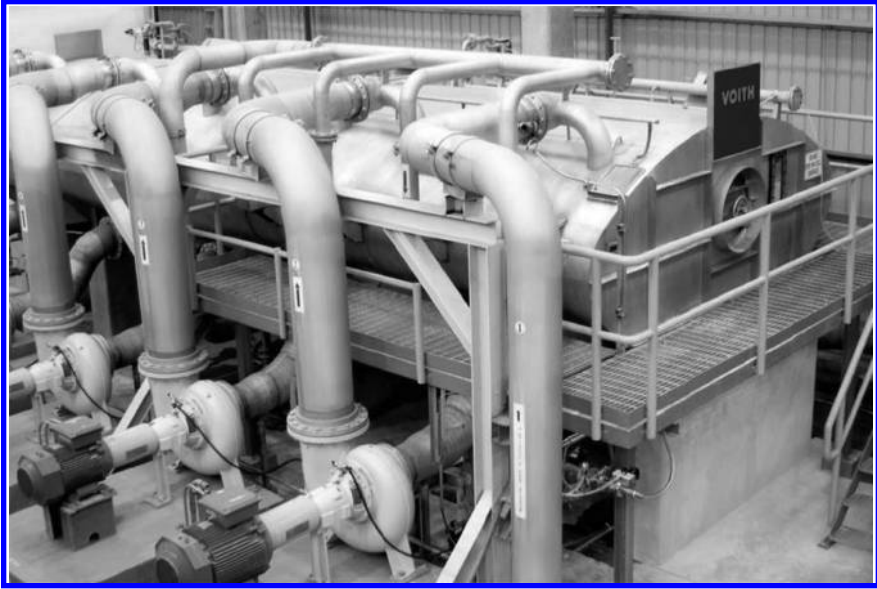
FIGURE 12.29 Photo of a typical deinking flotation cell. (Data from Voith Paper, GmbH & Co.KG, Heidenheim, Germany, 2014.)
