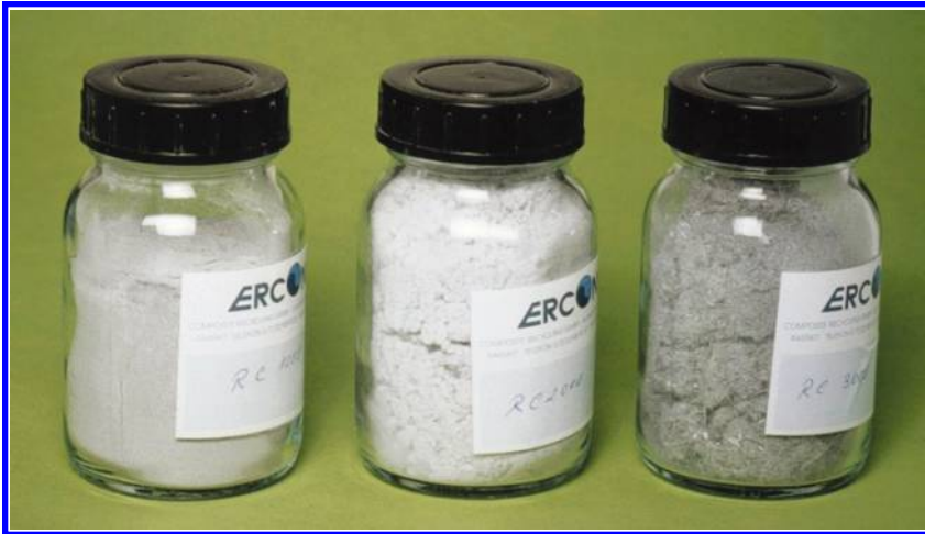
FIGURE 11.2 Fillers made from recycled composites by ERCOM. (Courtesy of M. Skrifvars.)
