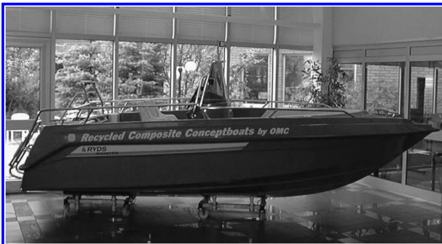
FIGURE 11.3 Motor boat made from 20 wt% recycled composite. (Courtesy of M. Skrifvars.)
