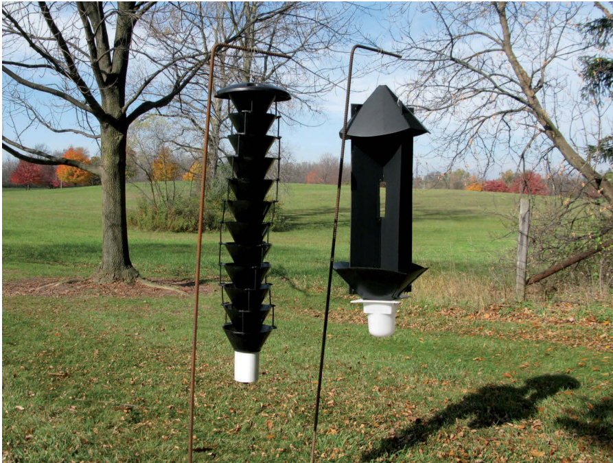
FIGURE 13.11 Types of pheromone traps that can be used for surveying cerambycidae. Left: multi-funnel trap; right: cross-vane trap. (Courtesy of Toby Petrice, USDA Forest Service.)
