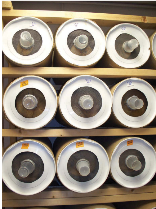
FIGURE 7.5 Cardboard tubes often used to hold infested wood until adults emerge. The lids have clear cups that let in light that attracts the adults and makes removing them easier. (Courtesy of M. Keena.)
