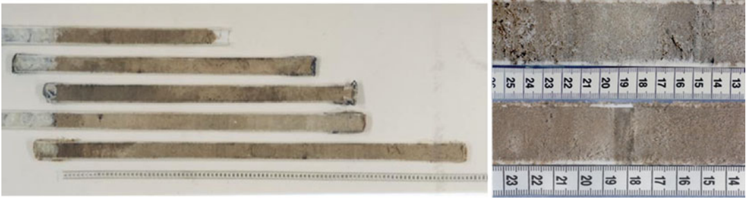
Fig. 3 Core samples from Umm Said Sabkha (Note that sand is dominant in the core sediments and microbial mats abundance in the third core)
