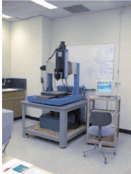
Fig. 29.6. Experimental CNC system — MHO MillRight Series 18 3-axis mill, with MDSI OpenCNC software controller. Custom PH curve interpolators can be invoked (in lieu of G code interpolators) by the macro capability of the OpenCNC software.
