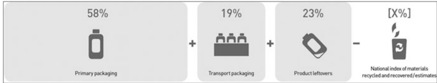
Fig. 8.16 Waste footprint breakdown according to life cycle stages for the Unilever portfolio for 2012. Potential amount of waste as defined before national adjustment (Source: Unilever 2013)
