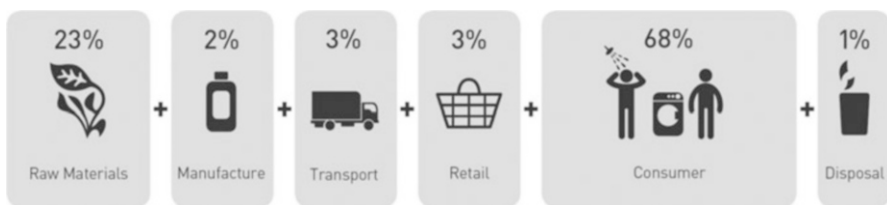
Fig. 8.14 Greenhouse gas footprint breakdown according to life cycle stages for the Unilever portfolio for 2013 (Source: Unilever 2014b )
