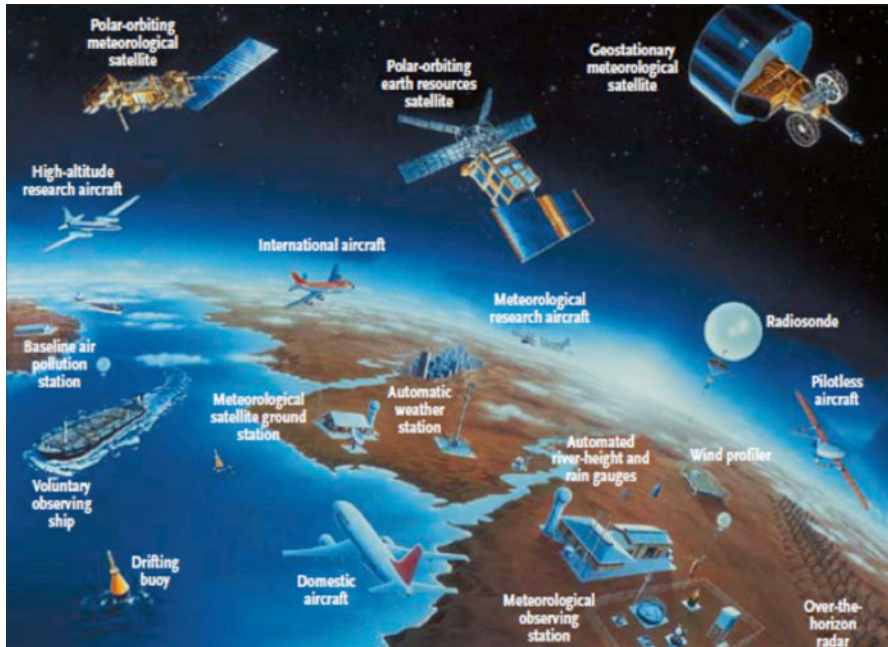
Fig. 6.1 Observing systems in use on the ground, at sea, in the atmosphere, and from space for monitoring and researching the climate system (WMO 2011)
