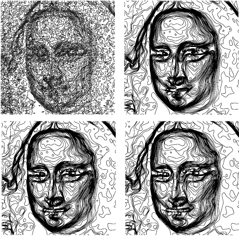
Fig. 6.38. Detail of "La Joconda". Top row. Left: level lines multiple of 5. Right: affine scale space. Bottom row. Left: mean curvature motion. Right: V = \kappa^2
