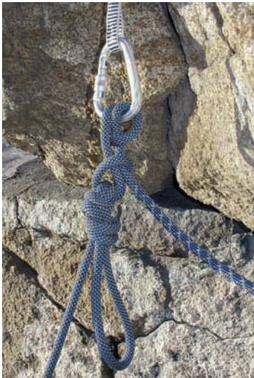
Figure 10.12 Tying the rappel line to a pear-shaped carabiner clipped onto the master point (using a Munter-mule combination with an overhand backup knot).
