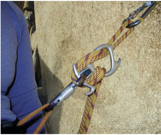
Figure 10.9 The Pirana is one style of a modified figure eight device that is often used in canyoneering.
