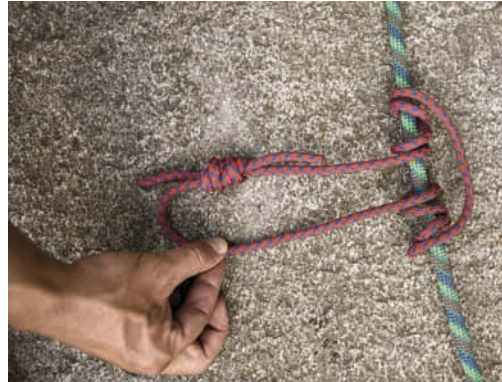
Figure 6.58 Getting ready to tighten by pulling a strand to the side of the fisherman’s.
