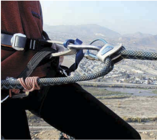
Figure 10.8 Make sure the brake side (or the rope going to the ground) is on the ground side of the rappel device when it's attached to your belay loop.
