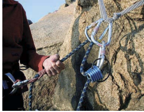
Figure 10.1 Mechanical device being used for lowering.
