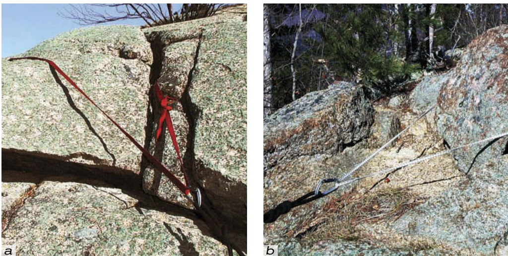
Figure 8.9 (a) Boulder with a good diameter and in a stable position, and (b) boulders too small and with an unstable position.
