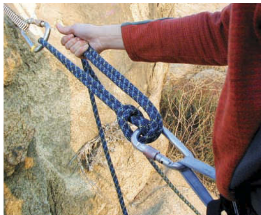
Figure 10.11 A Munter hitch can be used to rappel when you don't have a mechanical device.
