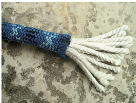
Figure 5.1 Kernmantle rope with core exposed and sheath around it.
