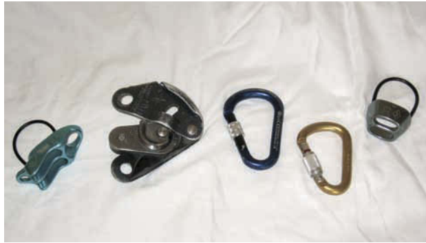
Figure 7.1 Examples of belay equipment (from left to right): Petzl Reverso, Petzl Grigri, Kong HMS, Petzl Attache, Black Diamond ATC.
