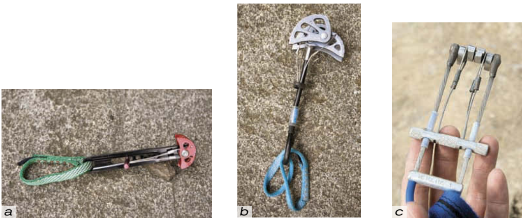
Figure 5.11 (a) Rigid stem, (b) flexible single-cable stem, and (c) U-stem (double) camming devices.
