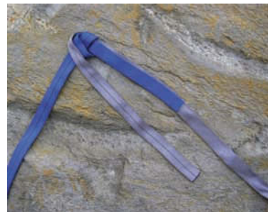
Figure 6.37 Second tail inserted in first overhand and pulled to about 12 inches (30.5 cm).
