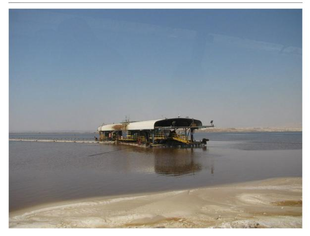
**Photo 9.5** The basis of the production process shown in Photo 9.4 is formed by differences in the solubility of natural salts depending on concentrations of brines. Water from the Dead Sea is delivered to ponds. As it evaporates, one or another salt precipitates. The retained water is drained off to the neighbouring pond evaporator, where there is crystallization of other salts by
