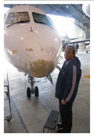
**Photo 3.27** Of all kinds of transportation, aviation is affected the most by hail. Hail blows break windshields and the surfaces of airplanes. They cause flight performance to deteriorate. This photo shows a Saab-340 airplane with windowpanes damaged by hail during a flight from Wellington to Napier. The pilot had to land at the airport of Palmerston North, North Island, New Zealand (Photo credit: *Manawatu Standard* newspaper, Palmerston North, New Zealand, June 2000)
