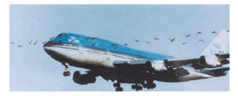
**Photo 5.115** With an aircraft speed of 555 km/h, a collision with a Canada goose (*Branta canadensis*; weight 6.8 kg) yields a force of 37,200 kg. The #1 engine on this KLM B-747 suffered an
