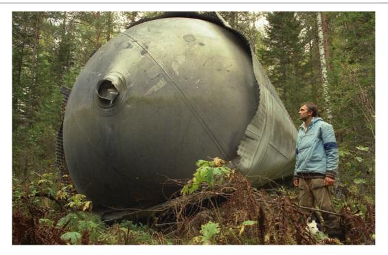
**Photo 13.30** The second stages of carrier rockets separate at altitudes of 140–160 km. Due to heating in the atmosphere, the fuel explodes when the stage is 25–30 km above sea level. Fragments fall to the ground, covering a large area. The fuel tank
