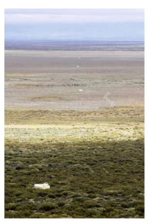
**Photo 7.10** This picture shows particle detectors. To reduce costs, the mesh of these particle detectors is rather coarse. They are located at a distance of 1.5 km from each other. The photo shows some of the water tanks displayed in Photo 7.9 (Photo credit: Karlsruhe Institute of Technology, Germany)
