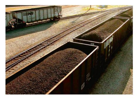
**Photo 12.7** The goods being transported themselves are sources of considerable pollution, which is caused by the leakage of those goods because of looseness; intensive emissions during loading, unloading, and transportation; and also by blowing-off
