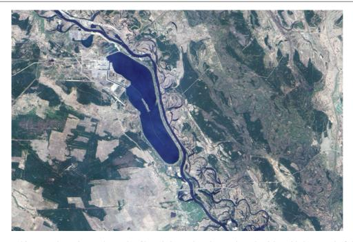
**Photo 8.11** This true-colour picture shows the Chernobyl nuclear power plant. The large body of water is a 12 km long cooling pond, and water channels run through the network of reactor-related buildings west of the pond. Reactor number four appears on the west end of a long building north-east of an
