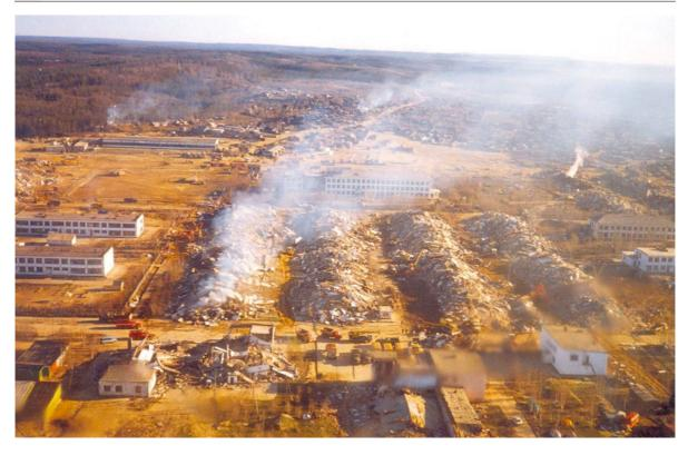
**Photo 1.2** The destructive character of the magnitude 7.5 Neftegorsk earthquake in Sakhalin on 28 May 1995 was caused mainly by the earth tremor. As a result, 17 of 22 panel five-storey buildings were completely ruined; two other buildings
