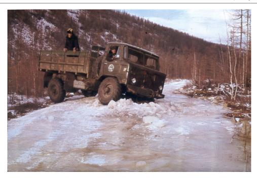
**Photo 2.25** Aufeises make roads slippery, which increases the number of road accidents. When an aufeis is not yet frozen on the top, cars bog down and freeze into ice if they stop. The photo
