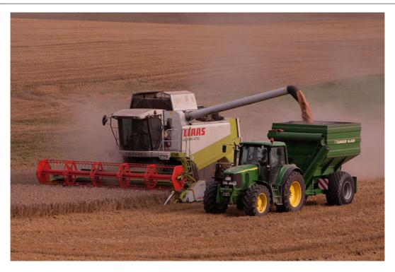
**Photo 11.5** The most environmentally important impact of plant growing is due to contact of soils with machinery. The ground is affected by the drive systems and operating parts of the agricultural equipment. By the end of fieldwork, only 10–15% of the agricultural land is not affected. The rest of the
