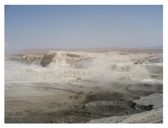
**Photo 10.3** Important sources of air pollution in opencast mining are motor transport and handling operations. The main component of atmospheric contamination is mineral dust. An
