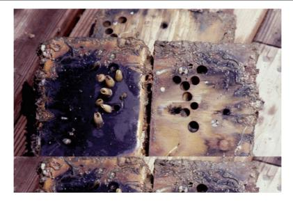
**Photo 5.126** The photo shows a timber section with internal damage caused by a marine borer (*Teredo*). This timber was exposed to marine borers at the US naval station in Honolulu, Hawaii; then it was lifted out of the water and split into two sections. White marks are calcareous sedi-
