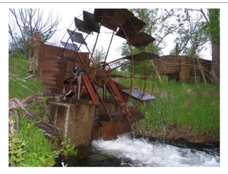
**Photo 8.4** In small water courses, hydroelectric stations designed to supply electricity to small power users in remote areas are not infrequently constructed. The photo shows one such
