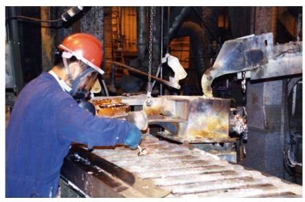
**Photo 9.19** In battery factories, the air is contaminated with dust containing lead, nickel, cadmium, arsenic, bismuth, antimony, and tin. The photo shows a worker who is ladling molten recycled lead into billets in a lead-acid battery recovery
