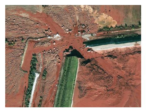
**Photo 9.15** Large amounts of toxic waste are characteristic of many enterprises in non-ferrous metallurgy. Accidents are frequent at their storage facilities. For example, such an accident occurred on 9 October 2010 at the aluminium plant in Ajka, Hungary. This is a natural-colour satellite image, showing the
