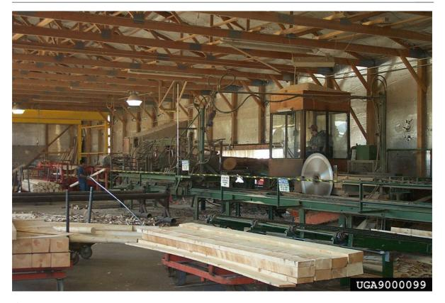
**Photo 9.23** Mechanical processing of wood is generally based on four working operations: (1) sawing, (2) planning, (3) drilling, and (4) polishing. As a result, sawn goods are produced that are used in construction, and manufacture of furniture, finishing
