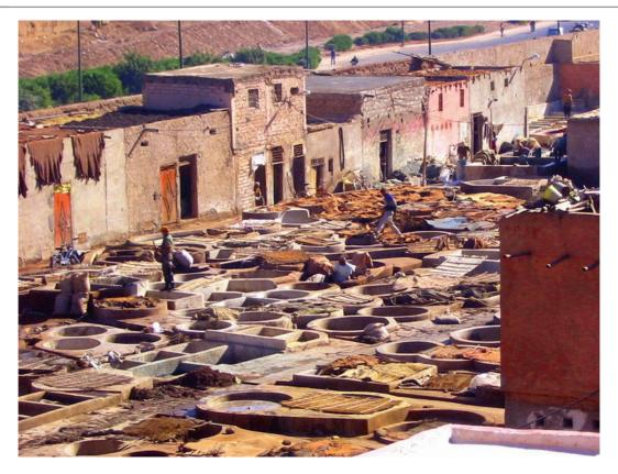
**Photo 9.31** The major contaminants in the tanning industry are chromium salts used for tanning, and cobalt, copper, and nickel, which are components of the colouring agents. In the treatment of 1 ton of raw stock, 200 kg of chlorides, 100 kg of
