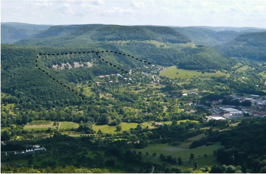
Fig. 3.8 Photo of study area taken facing north east. Lines indicate the boundaries of the landslide bodies
