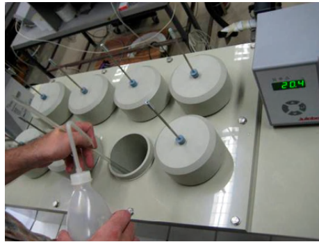
Figure 5.2. Sorption bench: pouring the salt solution into the containers
