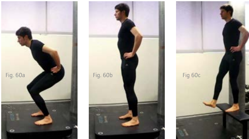
Fig. 60a-c: Starting position for jump tests in the standard jump test sequence: (a) squat jump, (b) counter movement jump, (c) drop jump
