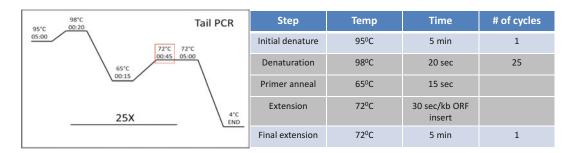
**Fig. 2** PCR setting for synthesizing DNA tailed template. Highlighted in *red* is the elongation step that must be set based on the size of the sequence insert. Elongation step requires 30 s per KB of ORF insert. PCR setting is based of manufacturer instructions from 2× KAPA HiFi HotStart ReadyMix kit
