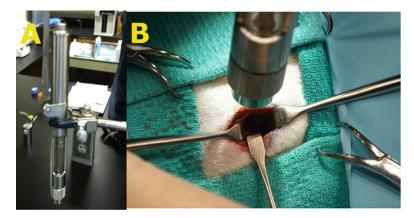
**Fig. 2** Needleless injection experimental setup in the rodent model. (**a**). The DermoJet<sup>™</sup> needleless jet injector mounted to an adjustable control arm. (**b**). The surgical field application demonstrating the injector aligned optimally for repeat safe injections toward the left ventricular surface area via thoracotomy access
