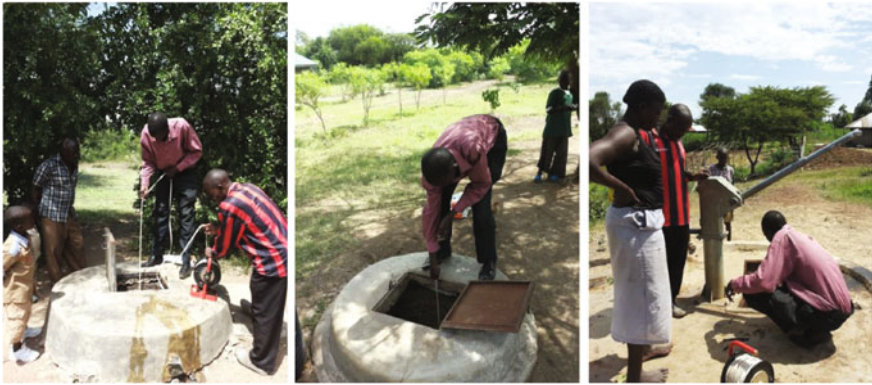
Plate 3 Measuring the water level in the shallow wells using an electric dipper
