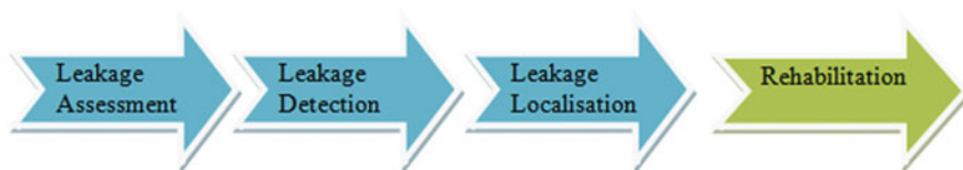
Fig. 1 Leakage management steps
