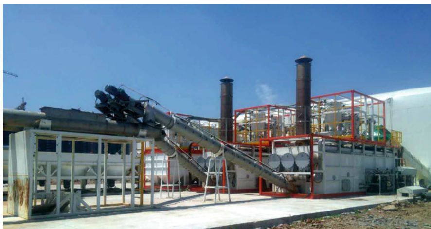
Fig. 4 Client, Hangzhou pesticide plant; pollutant type, organic pesticides; treatment capacity, 21T/H; treated quantity, 70,000 tons (December 2014)
