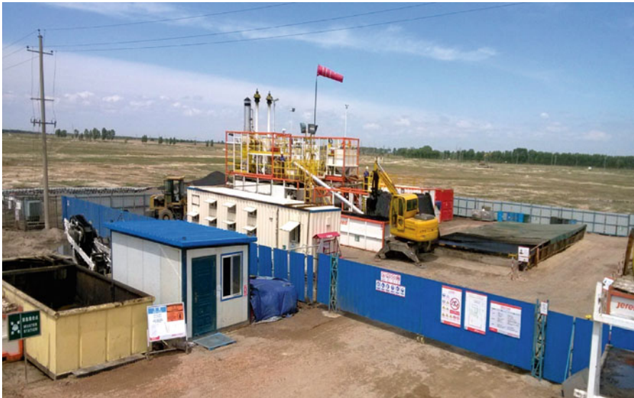
Fig. 2 Client, Daqing Oil Field; pollutant type, oil-based drilling cuttings; treatment capacity, 2T/H; treated quantity, 3,000 tons (August 2014)
