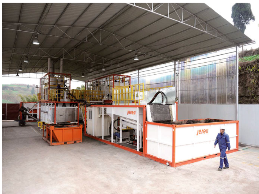
Fig. 5 Client, Sichuan oil-gas field; pollutant type, oil-based mud; treatment capacity, 2T/H; treated quantity, 2,000 tons (November 2014)
