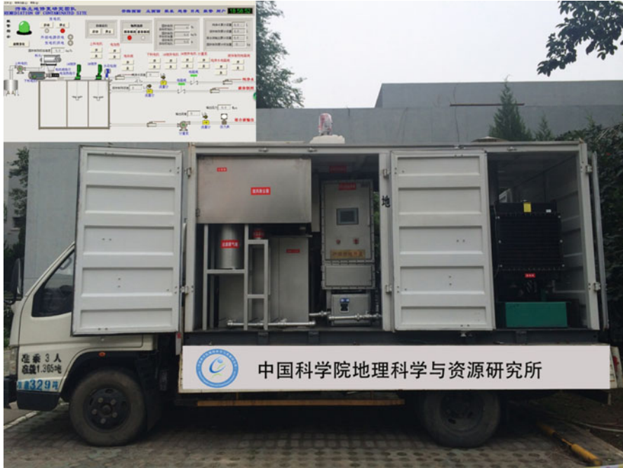
Fig. 2 Vehicle mounted and fixed oxidant injection equipment and its operating interface
