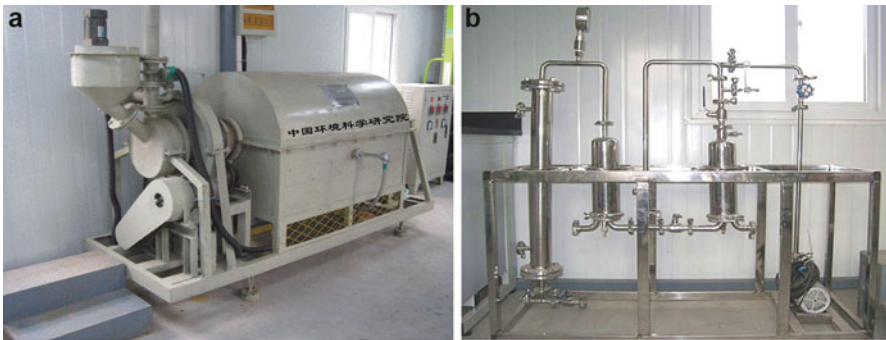
Fig. 7 Thermal desorption system. (a) Thermal desorption unit. (b) Off-gas treatment unit
