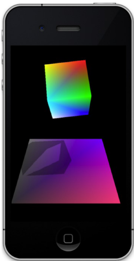
Figure 7-12. Z-fighting between the platform and the shadow
