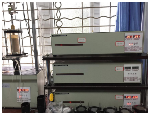
Fig. 7. Triaxial shear equipment
