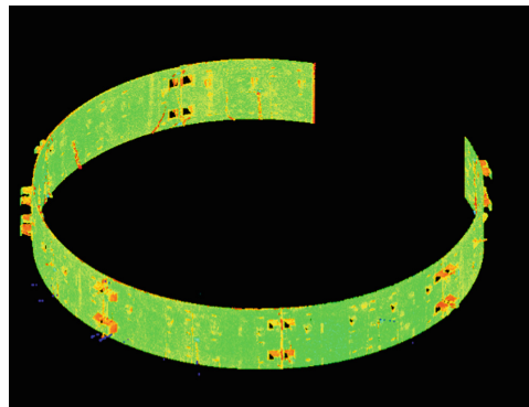
Fig. 13. Tunnel lining laser scanning data of one device before registration
