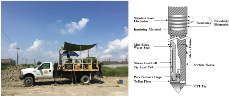
Fig. 2. Schematic diagram of field RCPTU test
