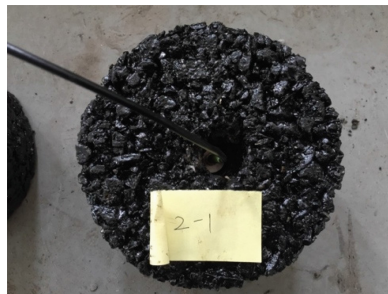
Fig. 2. Placement of high-precision optical fiber sensor
