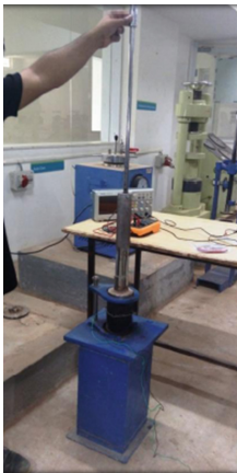
Fig. 7. Application of impact load bitumen specimens
