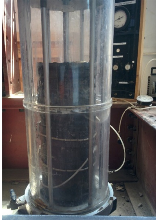
Fig. 1. 10-inch (255 mm) diameter specimen triaxial setup
