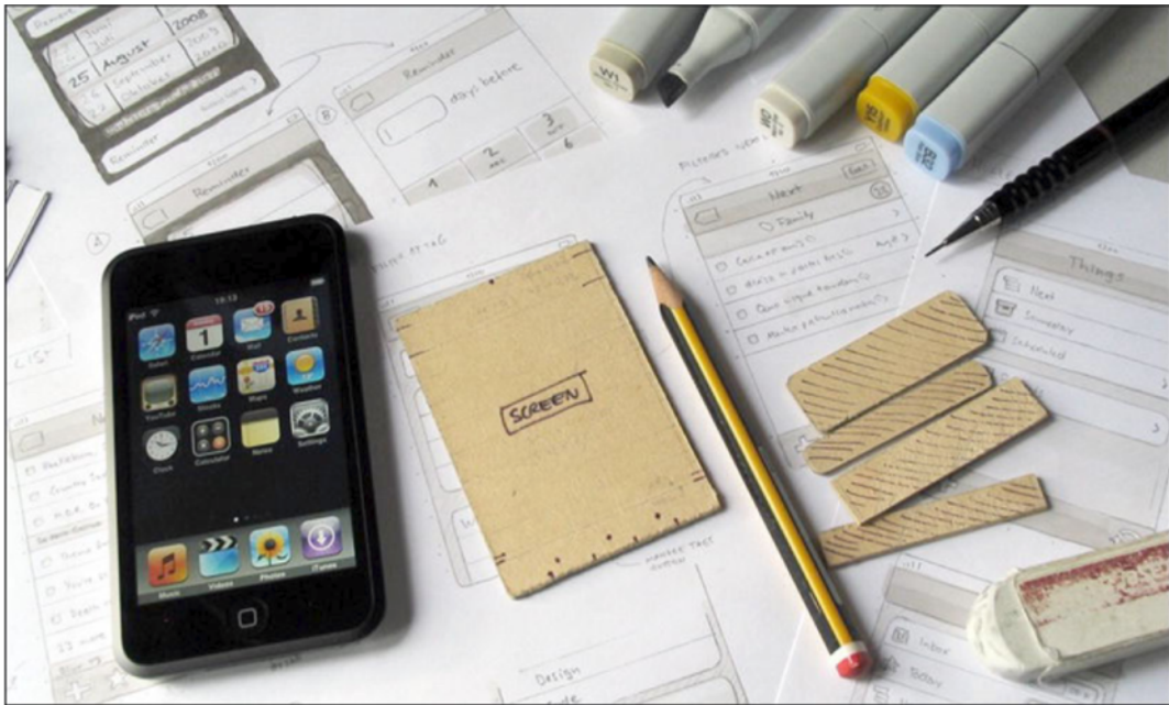
Figure 2–12. A handmade tool for drawing an iPhone or iPod wireframe (Image Cultured Code)
