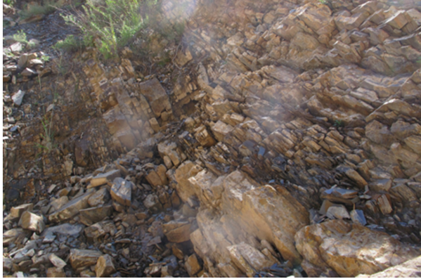
Fig. 3. Anti-dip layered rock mass of the slope toe.
