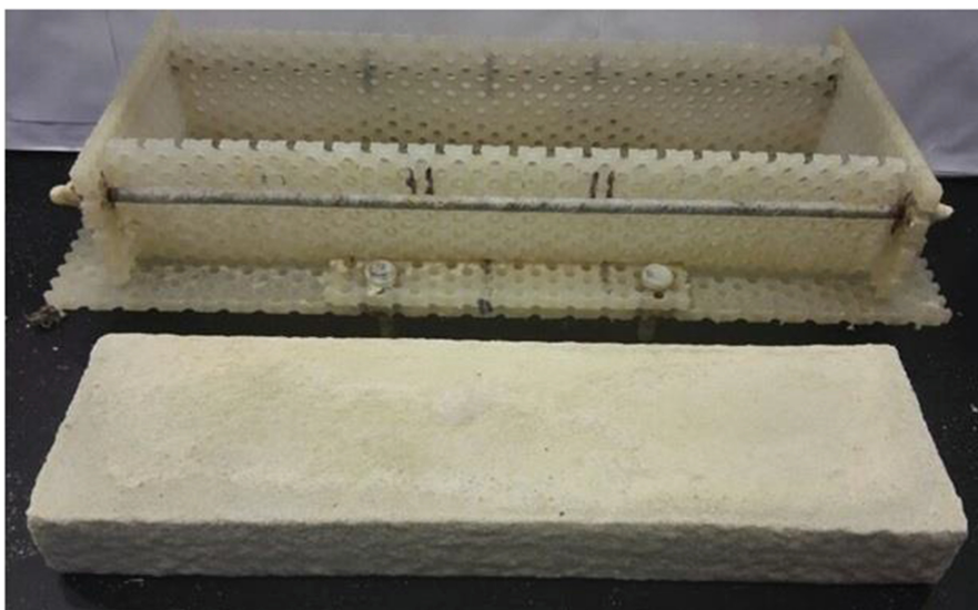
Fig. 1. Rigid full contact mold with image of one MICP-treated bio-beam. The bio-beam size is 355.6 mm \times 101.6 mm \times 38.1 mm (L \times W \times H).
