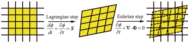
Fig. 1. The solving procedure of the CEL method.
