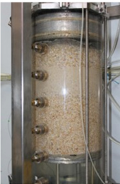
Fig. 3. Schematics and pictures of the filtration tests performed with oedopermeameter
