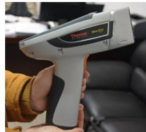
Fig. 2. Handheld XRF instrument
