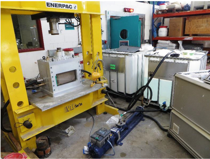
Fig. 2. Photograph of the layout of the high-pressure plane-strain sand production apparatus
