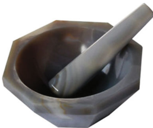
Fig. 2.3 Agate pestle and mortar used to grind rock samples. The diameter of this mortar is 10 cm, though many sizes are available
