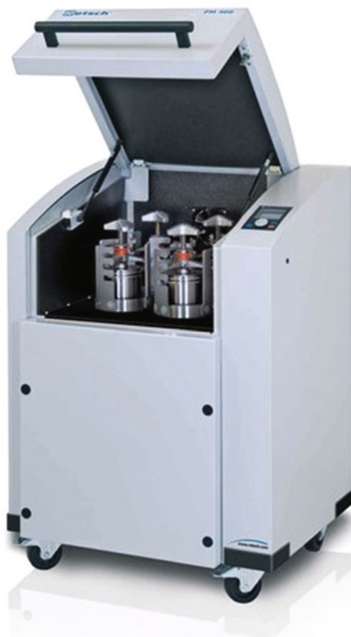
Fig. 2.2 Retsch planetary ball mill PM 400 used to micronize rock samples (after www.retsch.com )
