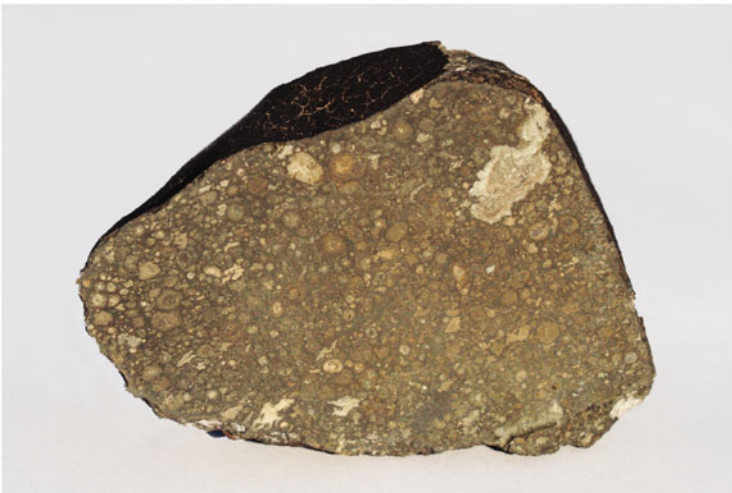
Fig. 6.2 Sawn surface of the carbonaceous chondrite Allende (CV3). The meteorite is composed of rounded chondrules, irregular shaped whitish Ca–Al-rich inclusions and FeNi metal grains all cemented by a dark carbon-rich matrix. Specimen is 7 cm wide
