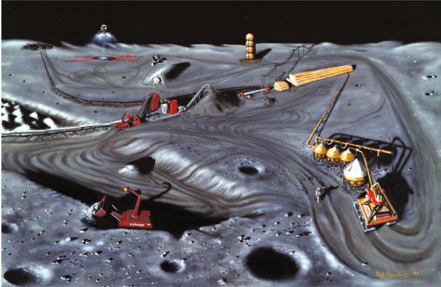
Fig. 15.6 Artist concept of a human settlement and surface mining operations on the Moon showing excavation, transportation, material handling, and processing equipment, as well as regolith covered habitats, roads, berms, launch pads, power lines, fuel depots, and communication antennas. Source: artwork by Pat Rawlings, painted in 1983
