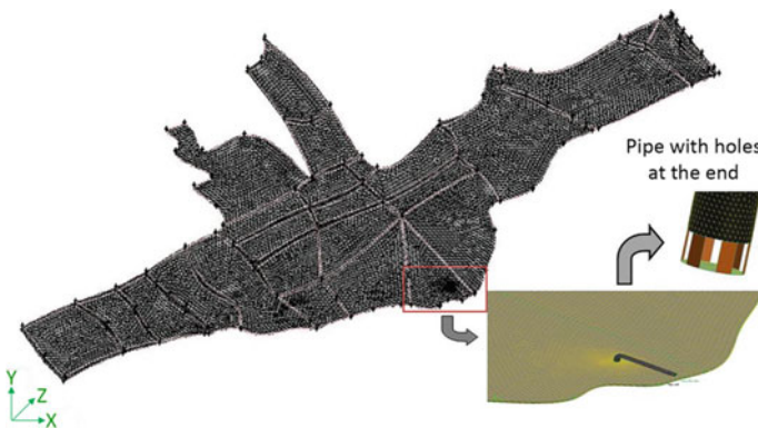
Fig. 18.6 A sample domain of lake and pipe with unstructured meshing (Shah et al. 2017)
