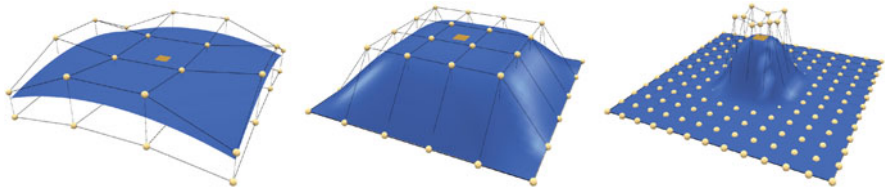
Fig. 10 Dependency of the deformation on the control lattice resolution. For all examples the same handle region was moved by the same translation
