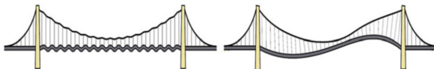
Fig. 1.9 Vertical ( left ) and torsional ( right ) oscillations in suspension bridges
