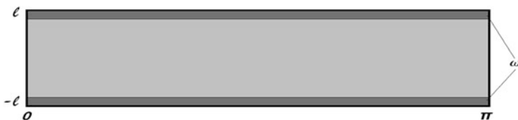
Fig. 5.3 The plate \Omega and its subset \omega (dark grey) where the hangers act
