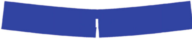
Fig. 5 Final crack situation at the end of the simulation after 10,000 SLA cycles [6]
