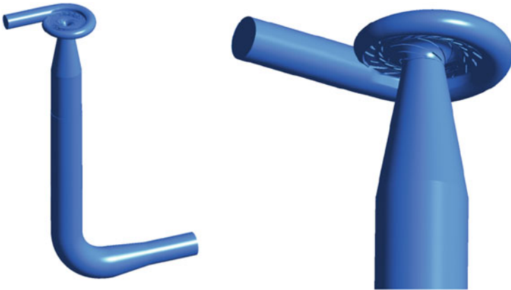
Fig. 10 Geometry used for flow simulations, the inflow is located top left at the spiral casing, overall height is \sim 4 m; left : complete geometry, right : detail
