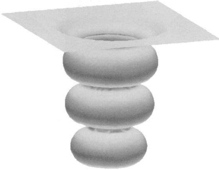
Fig. 42. Lithographic development on 50 \times 50 \times 50 grid.
