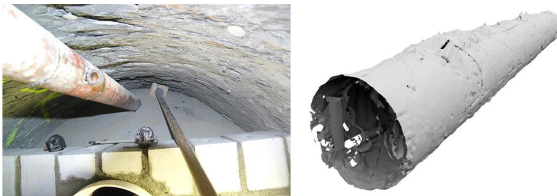
Fig. 5 Left Granular buffer emplacement using an auger system, right 3D image of the microtunnel test section before installation for volume calculation (Gaus et al. 2014)
