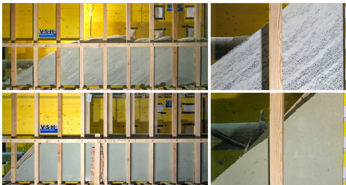
Fig. 14 ‘Fir-tree like’ segregation effects due to small material avalanches at the slope as seen in the second pre-test ( top pictures ) can easily be avoided by covering the slope, e.g. with a flexible mat ( bottom pictures )
