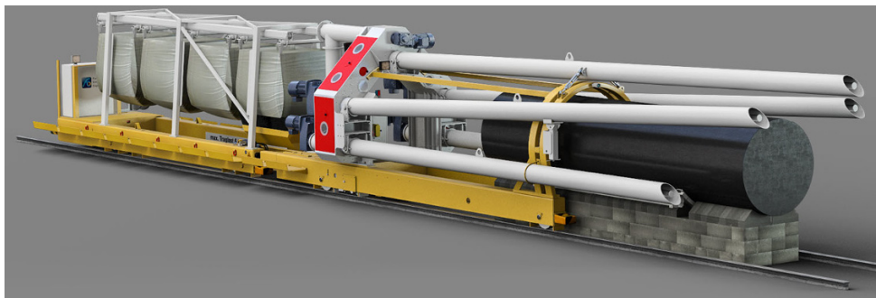
Fig. 15 Visualisation of the prototype ‘backfilling machine’ (BFM) with its five screw conveyors (driving over an approximately 1 m diameter canister on a bentonite block pedestal) developed for
