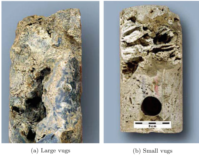
Fig. 1.17 A fractured rock domain with large and small vugs (Courtesy of Dr. George J. Moridis, LBNL)
