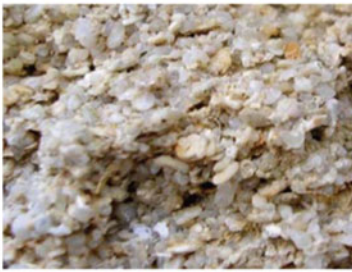
(c) High porosity sandstone
