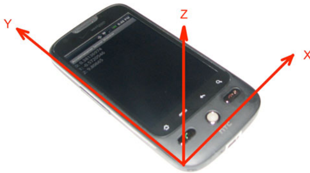
Figure 26–2. Accelerometer coordinate system
