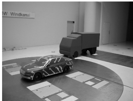
Fig. 2 Wind tunnel configuration in the case of overtaking process
