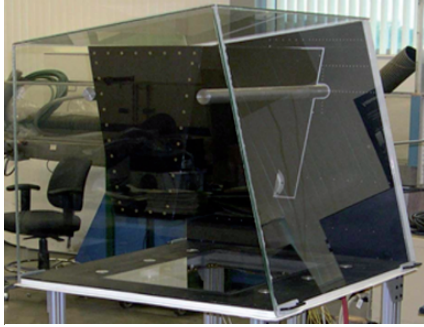
Fig. 1 Complete simulated underhood environment
