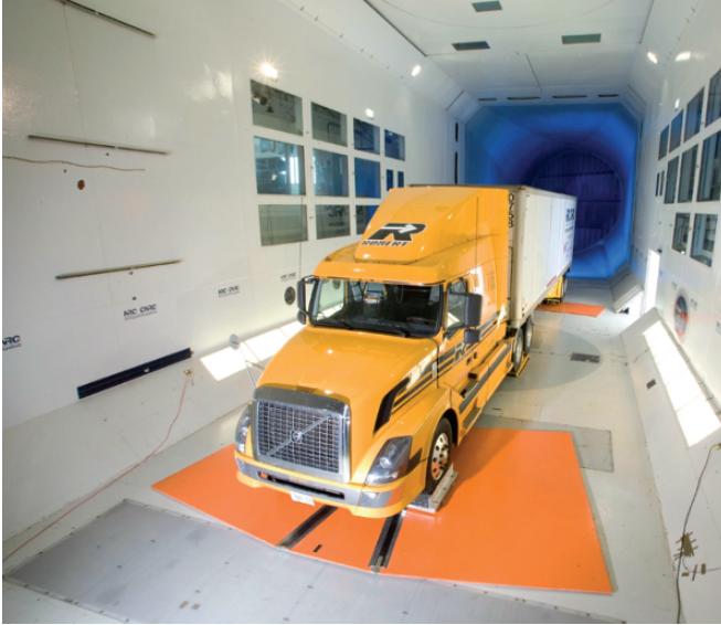
Fig. 1 Volvo VN 660 and 28-ft. Trailer in the NRC 9m x 9m wind tunnel
