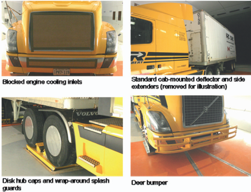
Fig. 3 Common components whose drag effects were measured
