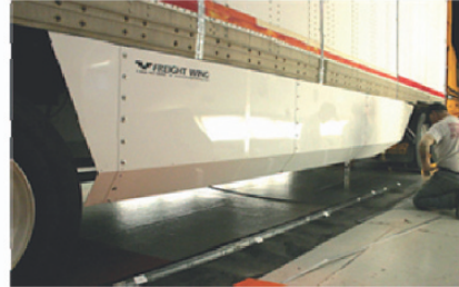
Freightwing belly fairing (low rider extension shown unattached)
