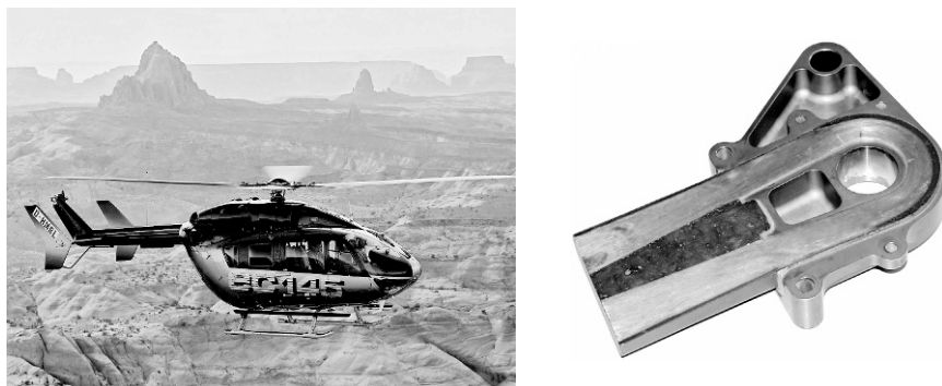
Fig. 2 The commercial EC 145 helicopter with the components glass fibre composite lug and titanium fitting
