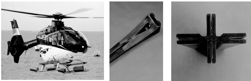
Fig. 5 The commercial EC 135 helicopter with the “flexbeam” main blade structure and torsion cross section
