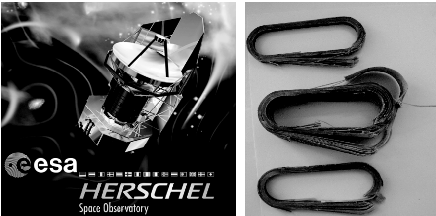
Fig. 4 Space Observatory HERSCHEL and liquid helium tank glass fibre composite support straps
