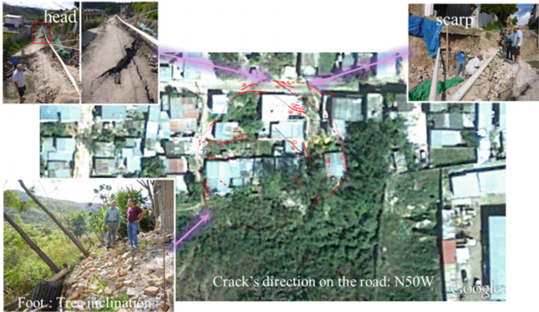
Fig. 5 The study site showing several displacements plotted in Google Earth and photos of the displacements
