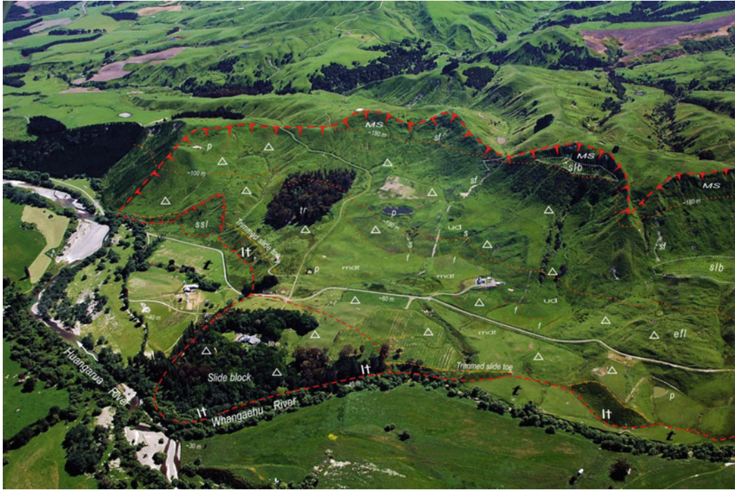
Fig. 4 Very large ( \sim 30 million m^3 ) complex of multiple landslides relict landslide near Martinborough (North Island, New Zealand). The larger relict landslide is thought to be several thousand years old, its main scarp (MS) is eroded, and its toe (lt) trimmed by the river when the terrace (t) was formed >1000 years ago. Field evidence suggests that the larger landslide periodically
