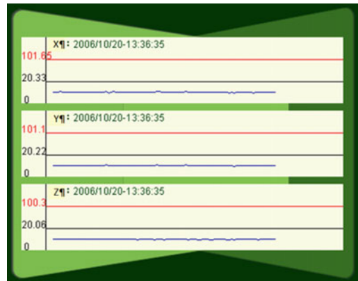
Fig. 5 Example of a geophone readout showing accumulated energy per second
