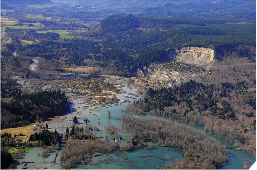
Fig. 45 This photo shows a recent example of a complex landslide. This landslide occurred in northwest Washington (USA) on March 22, 2014. Landslide debris covered about 40 homes and other structures as well as nearly a
