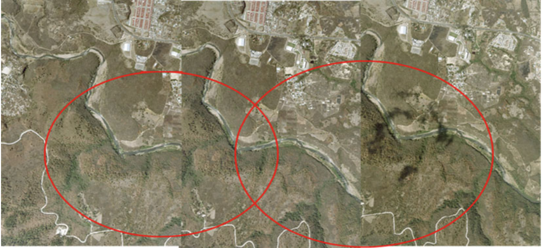
Fig. 13 Stereoscopic aerial photographs (digital aerial photos by JICA Honduras) of deep-seated landslide close to Choluteca River in Tegucigalpa, Honduras
