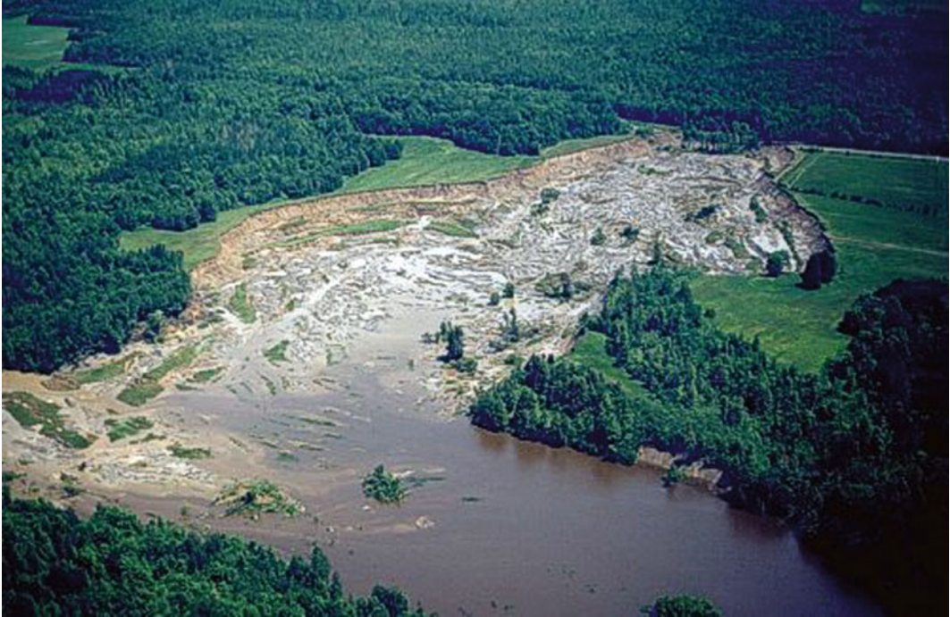
Fig. 34 The 1993 Lemieux Landslide was a rapid earth flow in sensitive marine clay near Ottawa, Canada. The headscarp retrogressed 680 m into level ground above the riverbank. About 2.8 million tons of clay and silt liquefied
