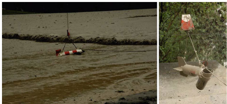
Fig. 12 Sampling device at Jiangjia Gou, China (density, concentration, rheological parameter)
