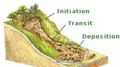
Fig. 1 The generation of a debris flow (courtesy of Prof. Hongey Chen and Soil and Water Conservation Bureau, Taiwan, http://246eng.swcb.gov.tw/ )
