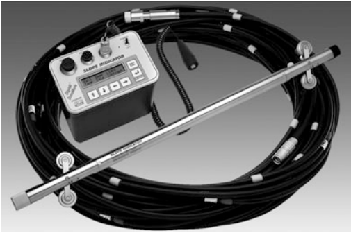
Fig. 3 The inclinometer probe (slope indicator)
