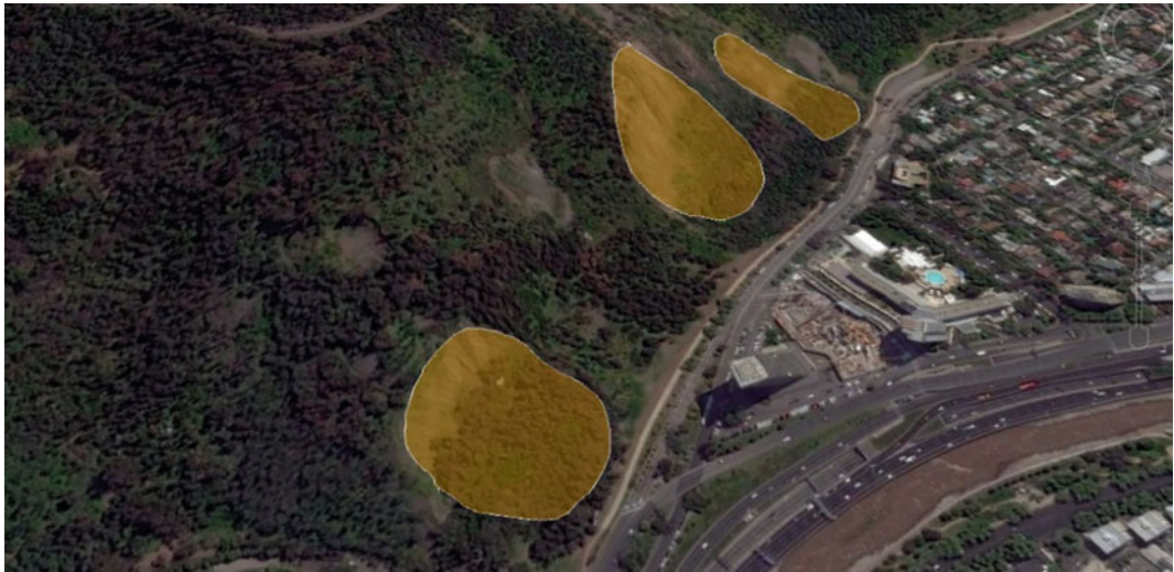
Fig. 19 Shallow landslides identified on Google Earth in Santiago, Chile
