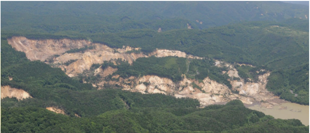
Fig. 16 The June 14, 2008 Aratozawa landslide in Japan is an example of rotational movement in the upper area of the headscarp and translational movement in the central and lower part. It can be typed as a Complex Landslide, since it includes more than one type of movement (Miyagi et al. 2010). This photo was taken by Fukuoka H. in 2008. See Figs. 44 and 45 for thematic illustration and photo of a Complex landslide
