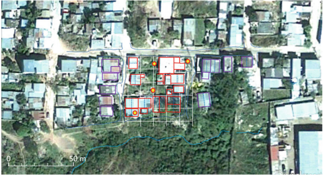
Fig. 7 Tracing the location of houses and roads before the landslide ( Red circles show drill holes, red-lined quadrangle indicates houses before the landslide (Google Earth on Dec. 10, 2010) )
