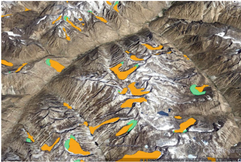
Fig. 17 More detailed identification of deep-seated landslides with scarps using Google Earth for the mountains in northeastern Afghanistan (Green-colored
