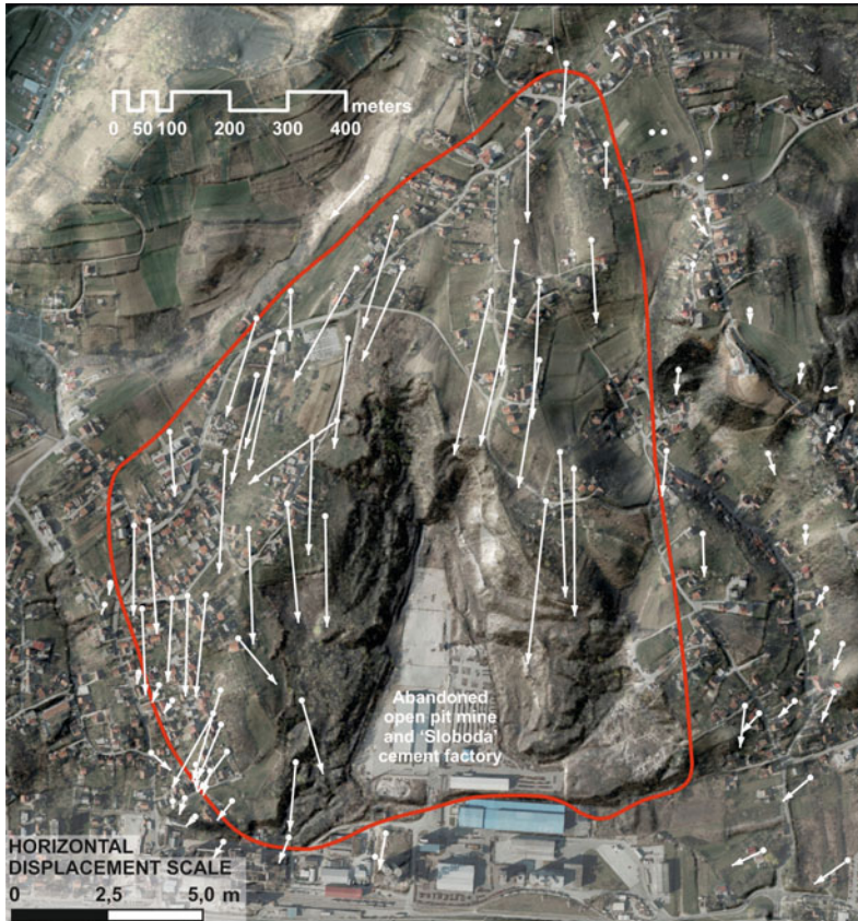
Fig. 1 Horizontal displacements ( white arrows ) at the Kostanjek landslide area in the period 1963–1988 based on interpretation of stereo pairs of aerial photographs from 1963, 1979, 1981, 1985 and 1988 (Ortolan and Pleško 1992). Red line depicts the outline of the Kostanjek landslide according to interpretation by Ortolan (1996). In the background are maps from March 2012:
