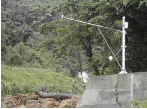
Fig. 6 Example of an ultrasonic water level transmitter
