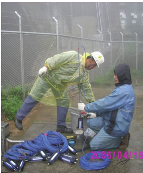
Fig. 10 Field installation of in-place inclinometers (DECL, Taipei, Taiwan)
