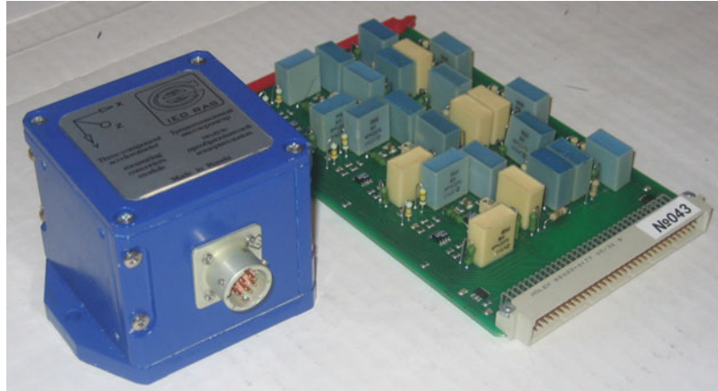
Fig. 7 Three-component accelerometer (primary converters module and frequency characteristic)
