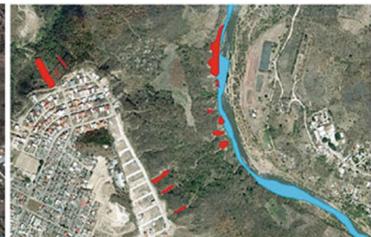
Fig. 18 Failure at steep slope in Tegucigalpa, Honduras. a Air photo from Google Earth 2013, b Air photo of digital aerial photo from the same year. Red areas in (b) are failures on steep slopes at Tegucigalpa city
