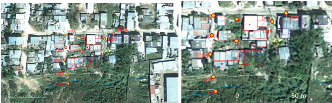
Fig. 10 Measuring: Left Level measuring points, Right an enlarged image of the left. Plot the level measuring points on the Google Earth image (brown colored circles: 5 m height, interval points set by level measuring)
