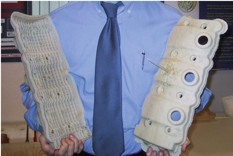
Fig. 10.5 Subsequent parts produced in polyamide 66 (30% glass fiber)
