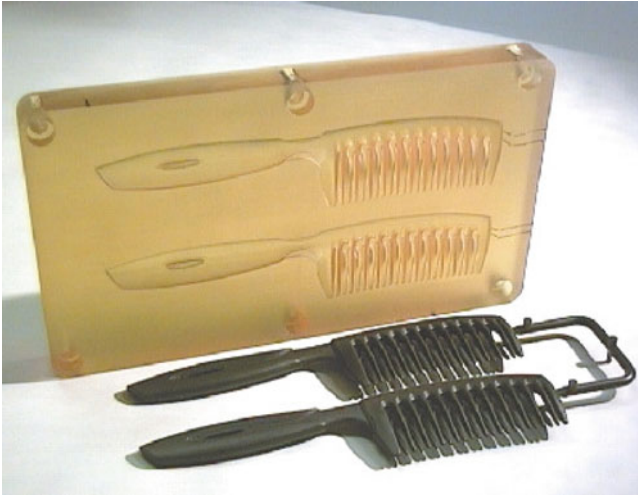
Fig. 10.1 Injection molding insert generated by stereolithography, shown with part
