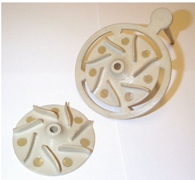
Fig. 10.3 PEEK impeller molded by stereolithography tools [21]
