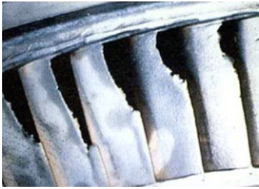
Figure 3: Solid particle erosion of the worn steam turbine blades.
