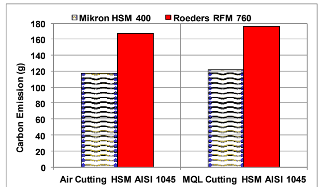
Figure 8: Carbon emission at high cutting speed of 32000 rpm.
