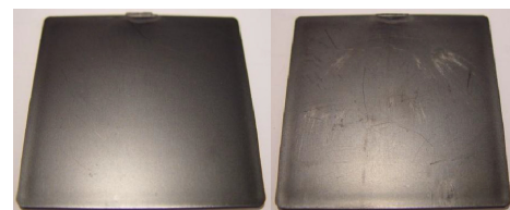
Figure 7: 100% recycled 0,25mm sieved (left) and non sieved (right) HIPS-PPE with PFR.
