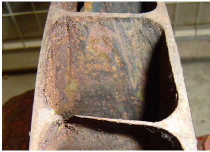
Figure 2: The thinning failure of erosive wear blades.
