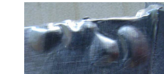
Fig. 8. Bulging on the rear of blade after shocking
