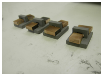
(b) Bronze material arrangements with "green" parts before being placed in furnace
