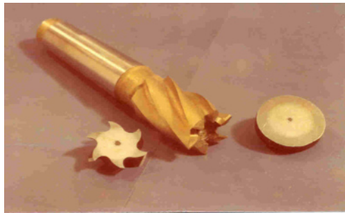
Fig. 8 General view of bimetallic end milling cutter and cross section of the initial bimetallic bar
