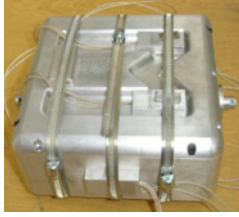
Fig. 2. Mould (300 mm by 300 mm by 80 mm deep) with Heaters attached
