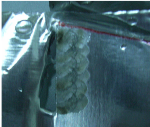
Fig. 5. Injured flank of blade due to rupturing Al foil
