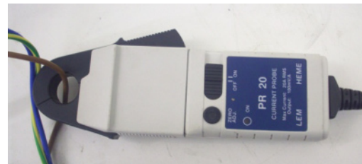
Fig. 7: LEM PR 20 Current Meter
