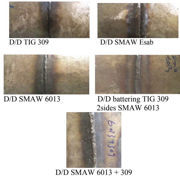
Fig. 4. Examples for similar welded specimens of ductile cast iron made by various welding procedures.
