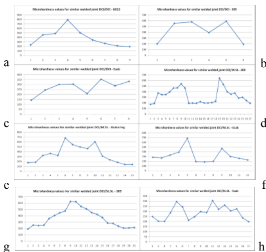
Fig. 8. Microhardness distribution along BM, FB, HAZ and WZ for similar and dissimilar welded joints.
