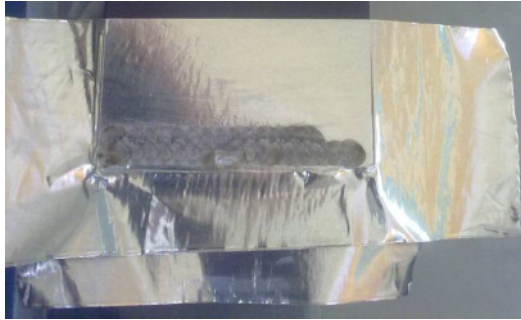
Fig. 4. LSP of double sides of blade with two Al foils
