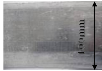
Fig. 4. Condition of the surface of as cast strip, thickness of this strip is 1.2mm.
