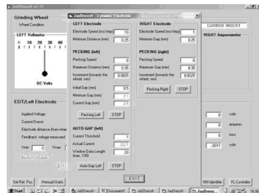
Fig. 2. Custom-built software to monitor and control the dressing
