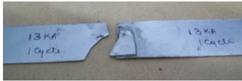
Fig. 13. Failure mode of weld-bonding specimen.
