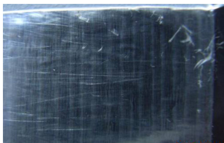
Fig. 9. The smooth and even surface of Al foil after scouring water on the rear surface of blade during LSP
