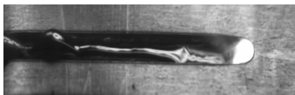
Fig. 7. Experimental observation of humps formation (courtesy of R. Fabbro, LALP)
