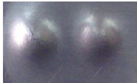
Fig. 7. Spallation on the rear of target
