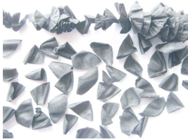
Fig 3: A sample of solid Neoprene chips produced using the cryogenic CNC machining process
