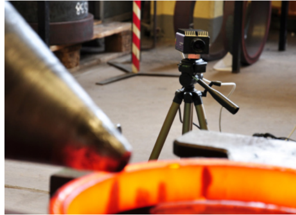
Fig. 4. Experimental setup: camera focussed on ring
