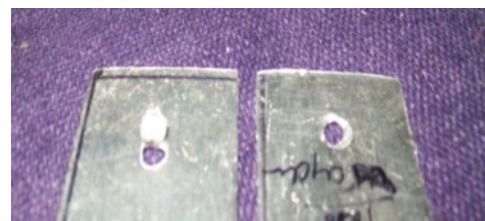
Fig. 12. Typical pictorial shows failure mode from nugget in spot welding during shear testing.
